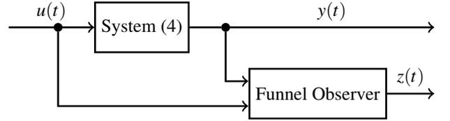
Figure 3: Interconnection of system (4) with the funnel observer (1).
