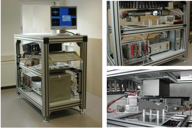
**Fig. 1** Picture of the PET-scanner 'PET-TW 05' Right: Front side with the integrated hardware components (above) and picture of the detector system (below)
