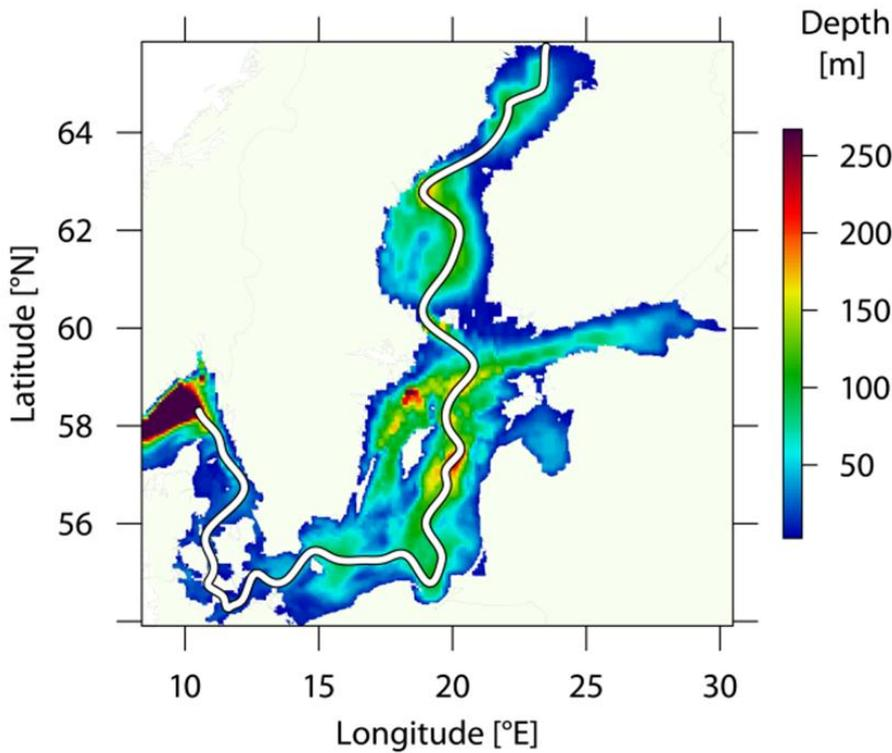
Figure 26. Overview of the chosen transect (white line) through the topographic map of the Baltic Sea model, which includes the main basins and sills.
