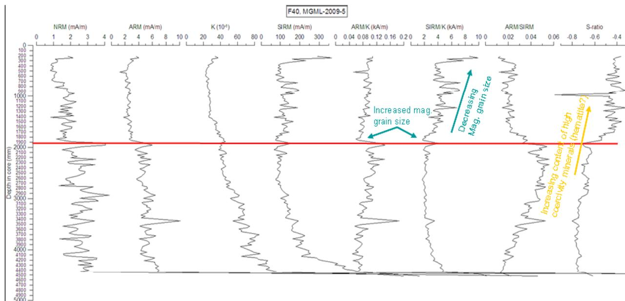
Figure 7. Mineral magnetic parameters determined for the core MGML-2009-5 from the eastern Gulf of Finland (F40 site). The red line indicates the erosional horizon at 190 cm.
