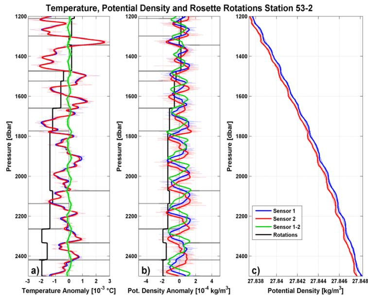
Fig. 3.3: Temperature (a), and Potential Density (b) anomalies. Blue: Sensor 1, red: Sensor 2, green: Difference Sensor 1 – 2. Black: Rosette rotations  $\times 0.2$ . Heavy lines: Band-passed anomalies showing only variability with length scales between 25 dbar and 250 dbar. Light lines: 1 dbar data. (c) Profiles of absolute Potential Density, with rotation-related wiggles clearly visible.
