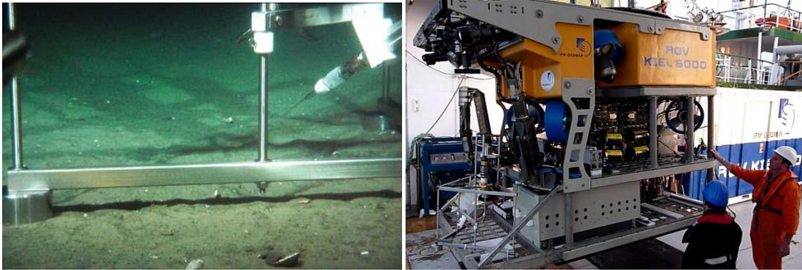
Fig. 5.3.1.1: Eddy Correlation (EC) Technique. Our EC system on the North Sea bottom (left) and on the ROV Kiel 6000 during the pre-deployment.
