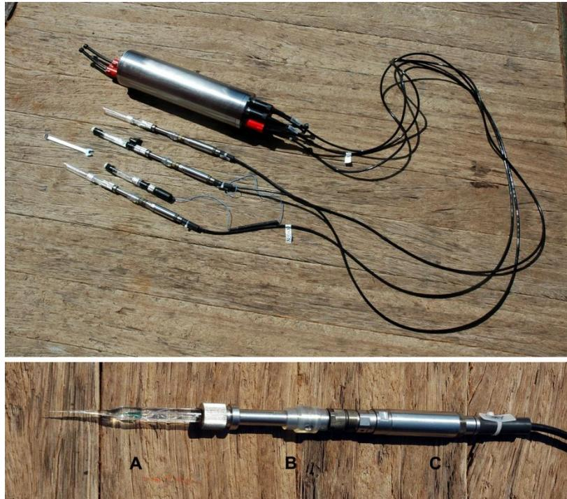
Fig. 5.2.1.2: upper panel, *in situ* micro-sensors connected to the data logging unit; lower panel, detail of *in situ* O<sub>2</sub> micro-sensor (A) connected to the amplifier (C) via an oil filled steel tube (B).
