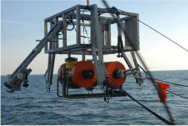
Fig. 5.2.1.3: Left: Video-guided deployment of the POZ-Lander with the launcher on top. The side view on the lander shows the ADCP (yellow) and the recovery items (flash, radio beacon and flag) in horizontal position.
