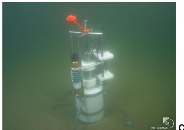
The Benthic Chambers (BC) are designed to measure benthic fluxes of dissolved chemical species over time at the sediment-water interface. They contain a cylindrical chamber (20 cm diameter)
