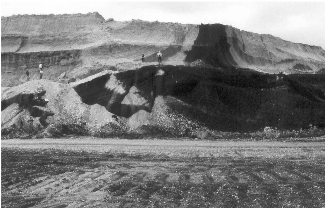
Fig. 3: Coal diapirism as an indicator of the deterioration of permafrost over large areas. South Profen Mine, 2005.
