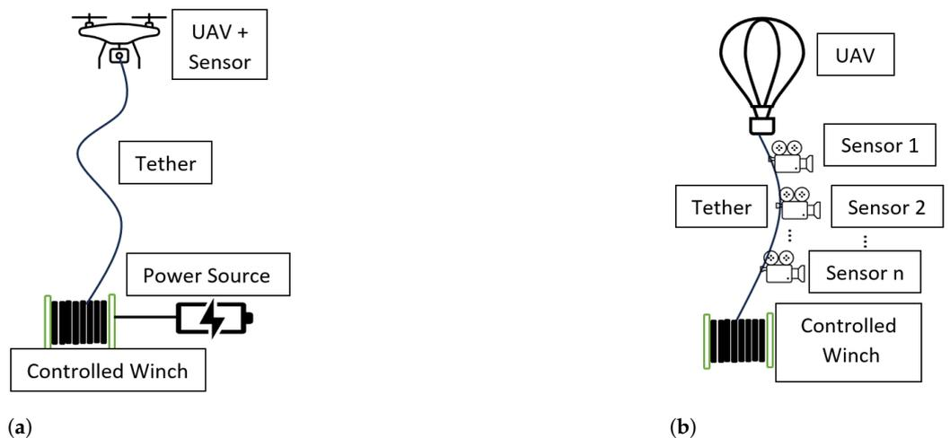
**Figure 8.** Examples of typical configurations in the meteorology application. (a) Sensor system on board the UAV. (b) Sensors distributed over the tether length.
