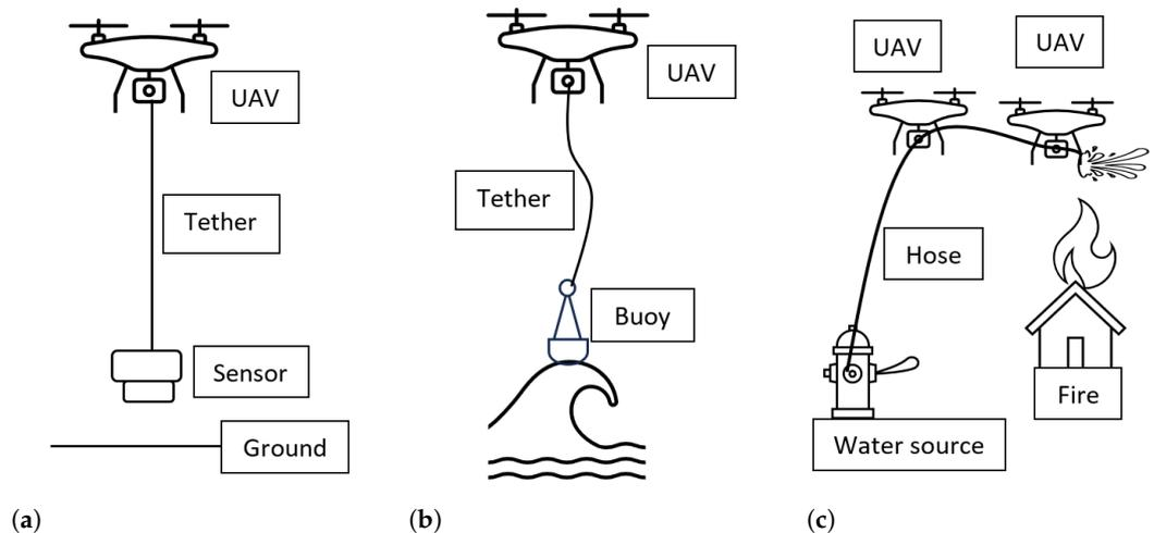
**Figure 7.** Examples of typical configurations in the load transportation application with different requirements: (a) Sensor transportation. (b) Buoy dragging. (c) Hose transportation.
