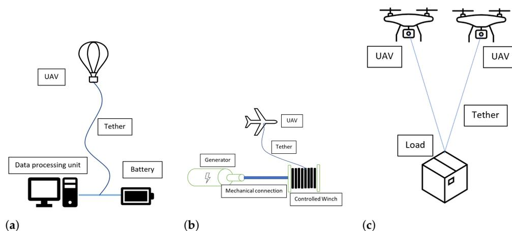
**Figure 1.** Typical configurations found in tethered UAVs for various application scopes. (a) Lighter-than-air UAV connected to a fixed point on the ground. (b) UAV used in wind energy harvesting. (c) UAV used to transport a load.
