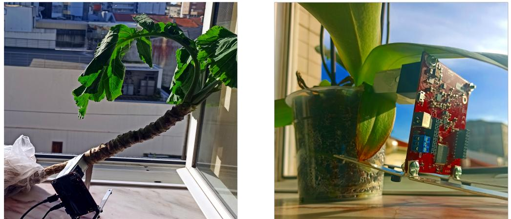
**Figure 8.** Radar setup to performs tests with a kale’s stem (**left**) and an orchid leaf (**right**).
