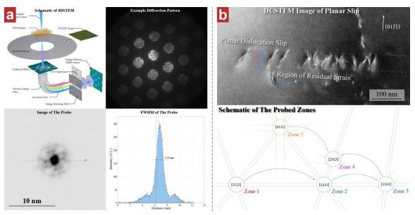
**Figure 1.** Beam condition and schematics of the multi-zone 4D-STEM strain mapping of a planar slip band (DAPB); (a), The electron probe from the patterned beam forming aperture; (b), Diffraction contrast STEM image of the interested planar slip and the Kikuchi map showing the associated zone axes.
