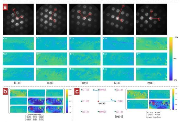
**Figure 2.** The local strain maps and reconstructed strain tensors; (a), The 2D strain maps of the slip band from 5 different orientations; (b), extracted full strain tensor of the area in a global Cartesian system; (c), The projected 2D strain tensor of [01-10] orientation.
