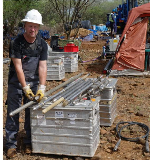
*Fig. 9.15: OSG slimhole wireline logging sondes at a drill site.*
