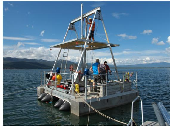
*Fig. 4.12: Platform for taking shallow piston cores*
