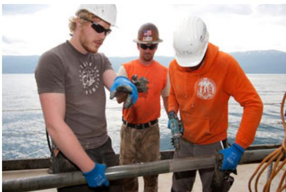
*Fig. 8.7: Drill core handling on the barge. Small holes were drilled into plastic liners to prevent excessive core expansion from high gas pressure in the liner (Photo: N. Leicher).*
