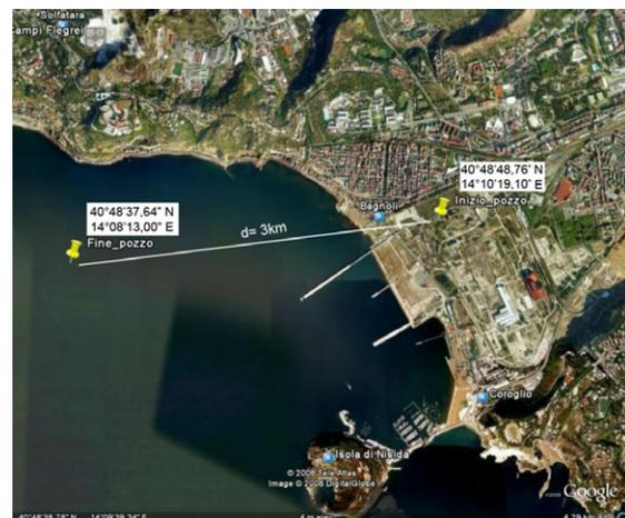
Fig. 5.9: Horizontal well trajectory for the Campi Flegrei drilling project in Italy
