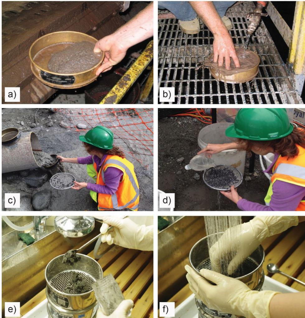
Fig. 8.17: (a) and (b) cuttings were separated from the liquids at the shale shaker and later washed with tap water (SAFOD); c) and d) cuttings were collected directly at the drilling mud outlet and rinsed later with tap water (DFDP); e) and f) chip size separation (< 2mm, 1-4 mm, > 4mm) and rinsing of cuttings after collection at the shale shaker (NanTroSEIZE).
