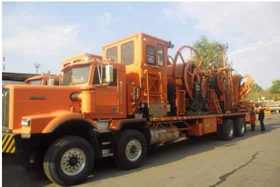
*Fig. 10.3: Truck-mounted coiled tubing unit (Wikipedia, CC BY-SA 4.0)*
