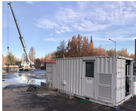
*Fig. 10.1: GFZ logging winch with 7000 m 7-conductor cable deployed in Otaniemi, Finland*
