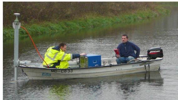
*Fig. 4.9: Shallow water survey with parametric sub-bottom profiler SES-2000 consisting of a transducer and a control unit and consuming less than 500 W (© Innomar Technologie GmbH 2006)*
