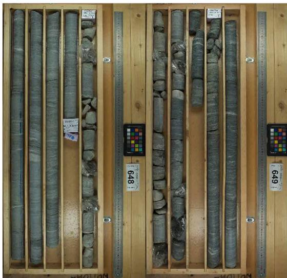
Fig. 8.4: Core boxes 648 and 649 from COSC-1. The core boxes are used in portrait format (=upper left corner = Top, lower right corner = Bottom). Top and bottom of core runs are marked with labelled foam blocks. Each box was photographed with the cm/ft ruler and a standard colour chart.
