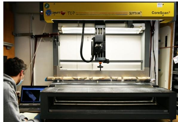
*Fig. 11.14: Optical core scanner in operation*
