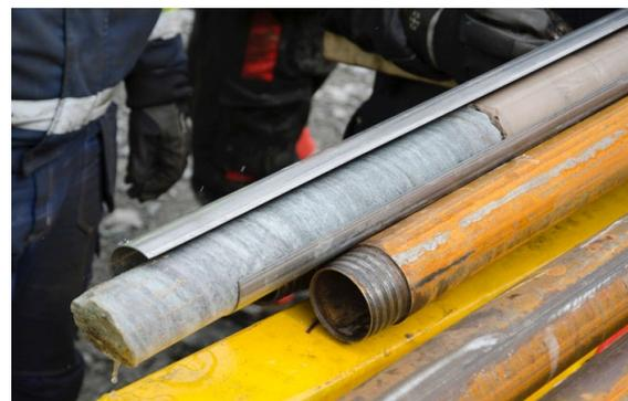
*Fig. 8.1: First COSC drill core (gneiss below cement) in opened inner tube of a triple tube core barrel assembly. Clearly visible is the split aluminium liner protecting core from external forces, the second tube, and the drill string tube, hence 'triple tube'.*
