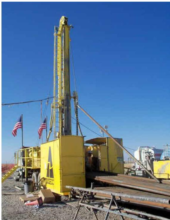
Fig. 5.2: Truck-mounted wireline coring rig at Snake River Plain (Project HOTSPOT)
