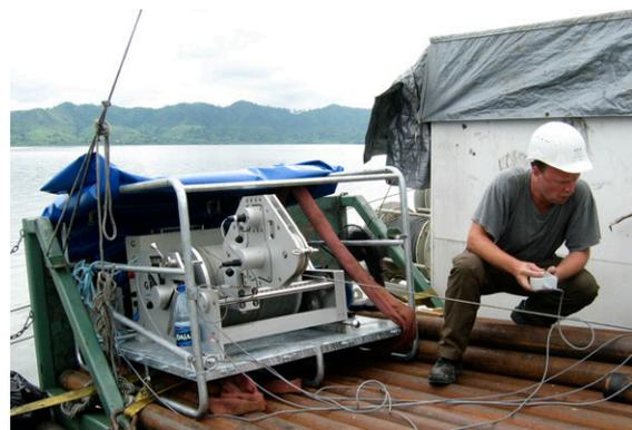
Fig. 9.13: Logging winch with 2.2 km of a 4-conductor cable.
