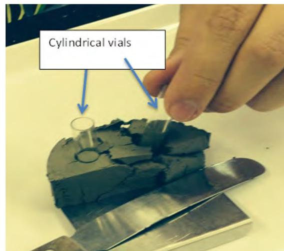
Fig. 4.5.11: Sub-sampling of a 2 cm-thick sample slide using cylindrical vials. The latter collect pre-defined volume samples parallel to the long axis of the core in a top to bottom direction, which enables the calculation of the water content, and thus dry and wet bulk density, respectively.
