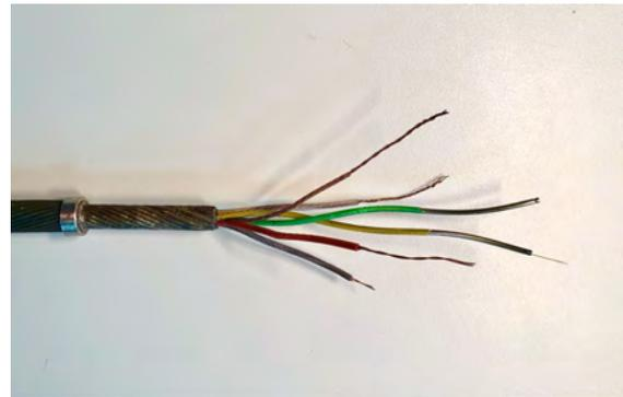
*Fig. 4.7.2: Armored wireline cable with 4 electric and 2 steel tubes holding optical leads*
