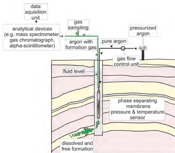
Fig. 4.7.9: Mode of operation of Gas-Membrane Sensor (GMS) and experimental workflow
