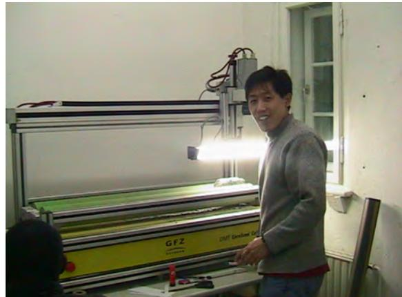
*Fig. 5.10: Optical core scanner in operation*
