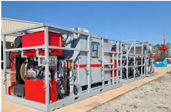
Fig. 4.7.3: Skid-mounted coiled tubing unit (Wikipedia, CC BY-SA 4.0)
