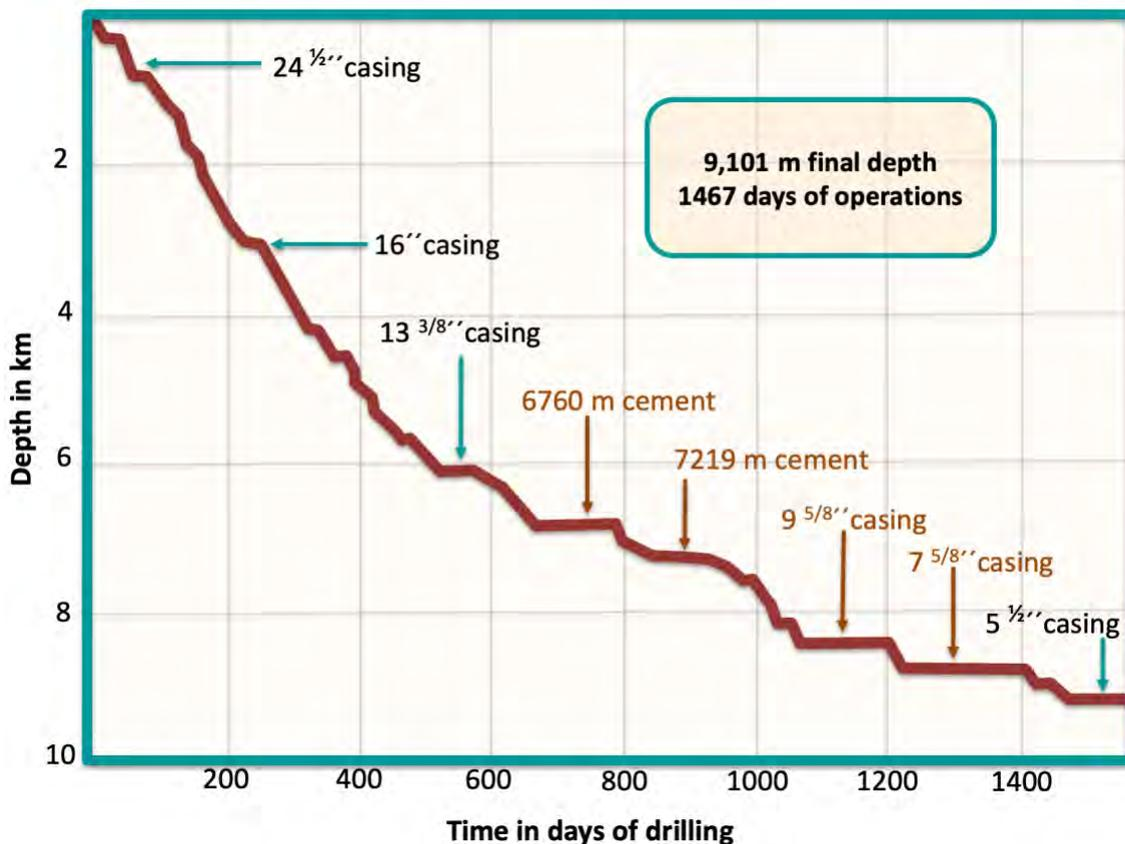
Fig. 3.4.1 Depth versus duration of drilling for the KTB well in Germany. Note that duration and costs are directly correlated. Major delays marked with brown arrows caused major cost increases.
