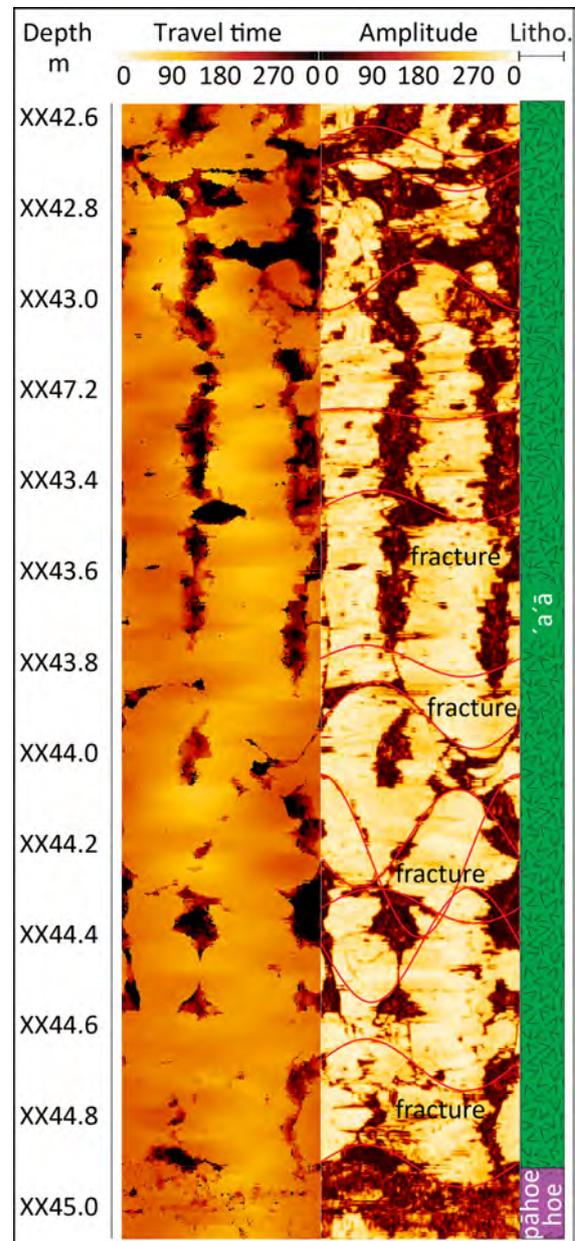
Fig. 4.6.12: Fractures on an acoustic image log
