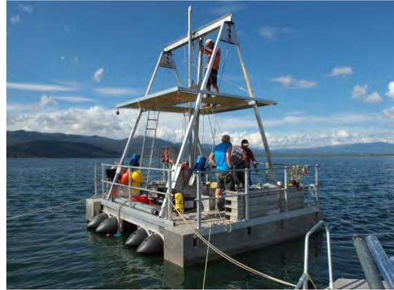
*Fig. 4.1.12: Platform for taking shallow piston cores*
