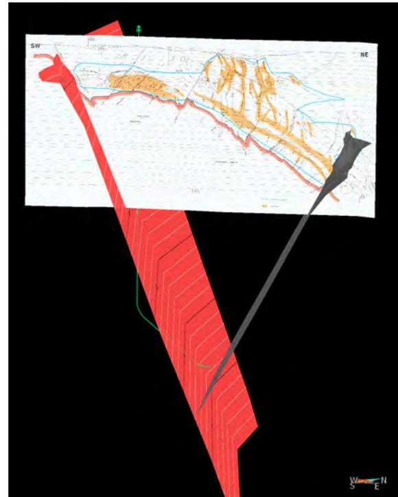
Fig. 4.2.8: Fault (red, grey) visualization in geologic section with well path (green) of Schneeberg-1 research well (courtesy: LfULG, State of Saxony)
