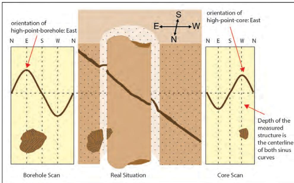
Fig. 4.6.7: Comparison of structural features in borehole wall images (left) and core images (right)
