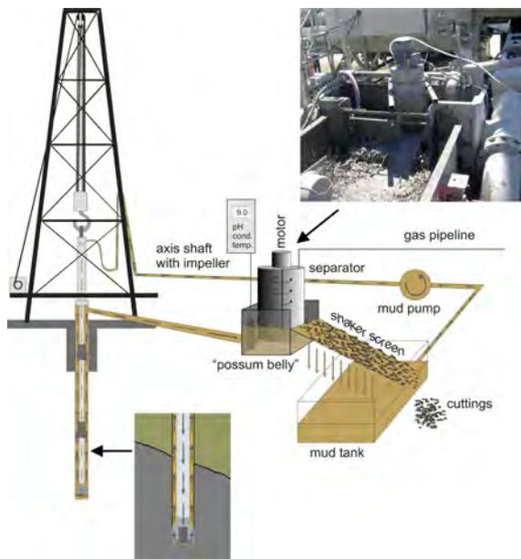
Fig. 5.11: Scheme of drill mud flow and gas extraction by gas separator; inset photo shows gas separation device
