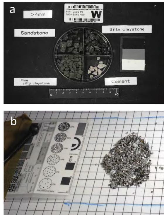
Fig. 4.5.19: Photographs of a) NanTroSEIZE cuttings (> 4 mm) separated in sandstone, silty claystone, fine silty claystone, and cement (from casing). The label in the upper part shows the expedition, drill site, drill hole, material number, method (solid taken from mud water), and the working portion; b) DFDP cuttings (all grain sizes) with percentage of area, sorting, roundness etc. for later description.
