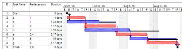
Fig. 3.2.3: Gantt chart example to show tasks, duration, and timing (Source Wikipedia)
