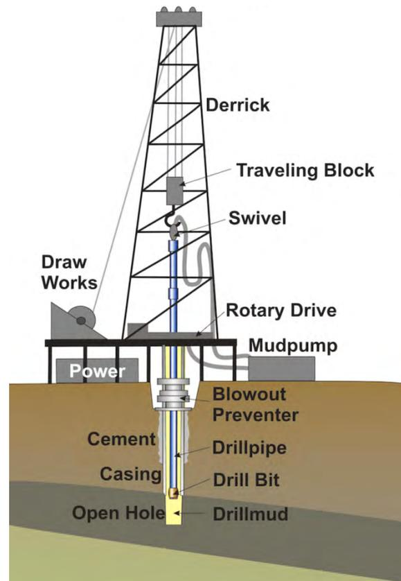
Fig. 4.2.1: Key components of rotary drilling
