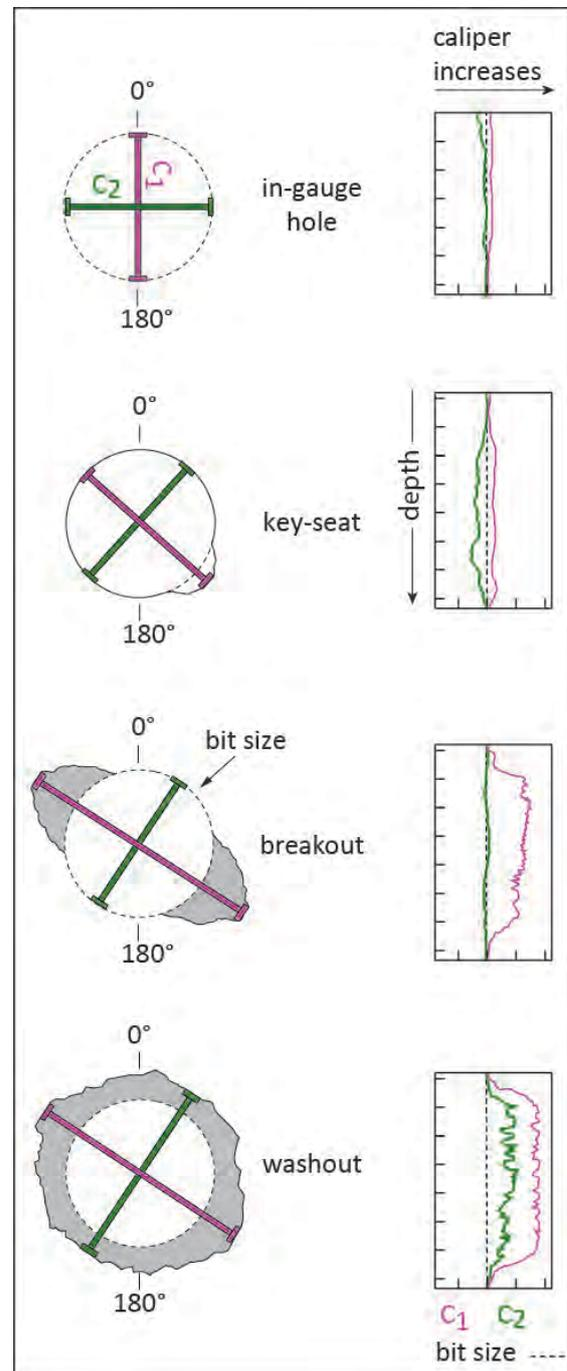
Fig. 4.6.9: Sketch of borehole size and shape (left column) and the corresponding caliper curves (right).
