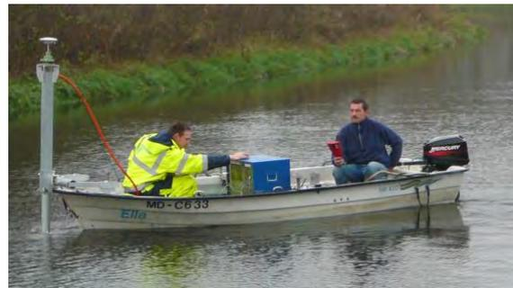
*Fig. 4.1.9: Shallow water survey with parametric sub-bottom profiler SES-2000 consisting of a transducer and a control unit and consuming less than 500 W (© Innomar Technologie GmbH 2006)*
