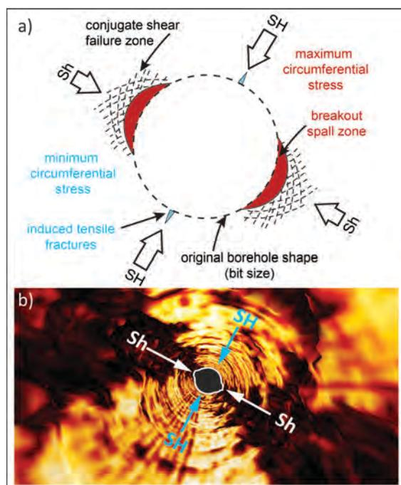
Fig. 4.6.10: Borehole breakout shape. a) In vertical holes breakout zones develop at diametrically opposing sides with the long axis of the elliptical zone parallel to the orientation of the minimum horizontal principal stress ( $S_h$ ). Perpendicular to the long axis, induced tensile fractures can appear and their orientation is parallel to the maximum horizontal principal stress ( $S_H$ ). b) 3-D borehole breakout view from ABI image of the borehole wall.
