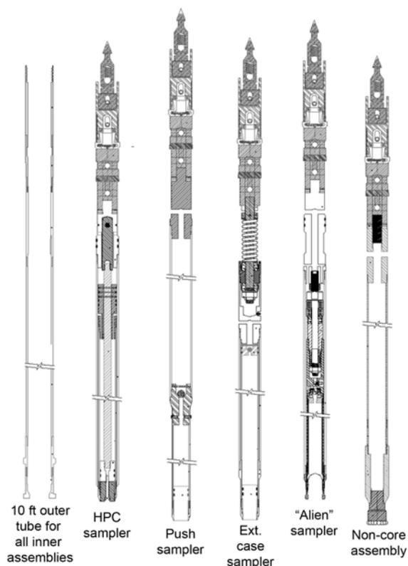
Fig. 4.2.5: Tools used for coring lake sediments
