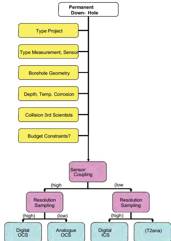
Fig. 4.7.8: Decision strategy for the design and selection for a typical PDM system
