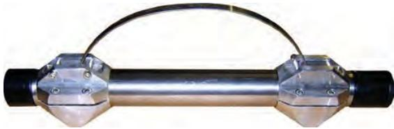
Fig. 4.7.4: Spring bow de-centralizer hole lock concept (photo: SAFOD project)
