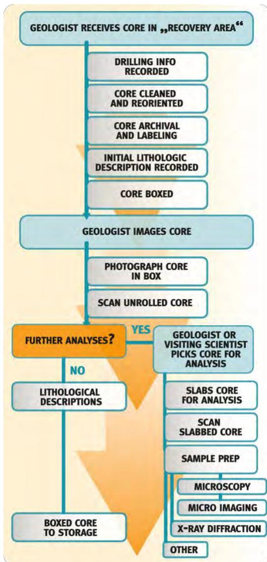
Fig. 3.6.3: Core handling protocol
