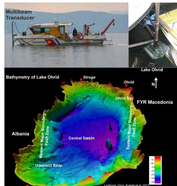
Fig 4.1.8: Upper left: Multibeam transducer mounted at the bow of a small survey vessel. Upper right: Details of the multibeam transducer. Lower part: Bathymetric map of Lake Ohrid collected with a multibeam system (taken from Lindhorst et al., 2012)
