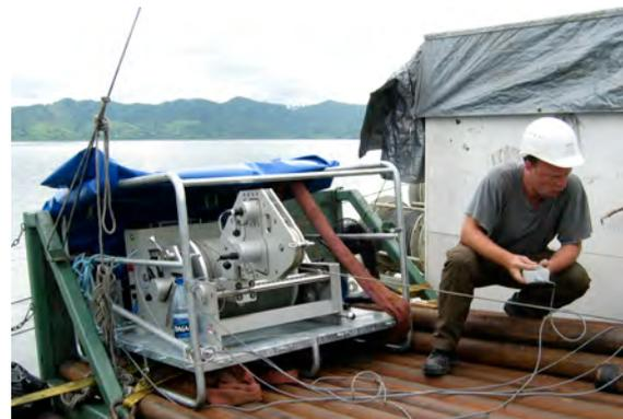
*Fig. 4.6.13: Logging winch with 2.2 km of a 4-conductor cable.*
