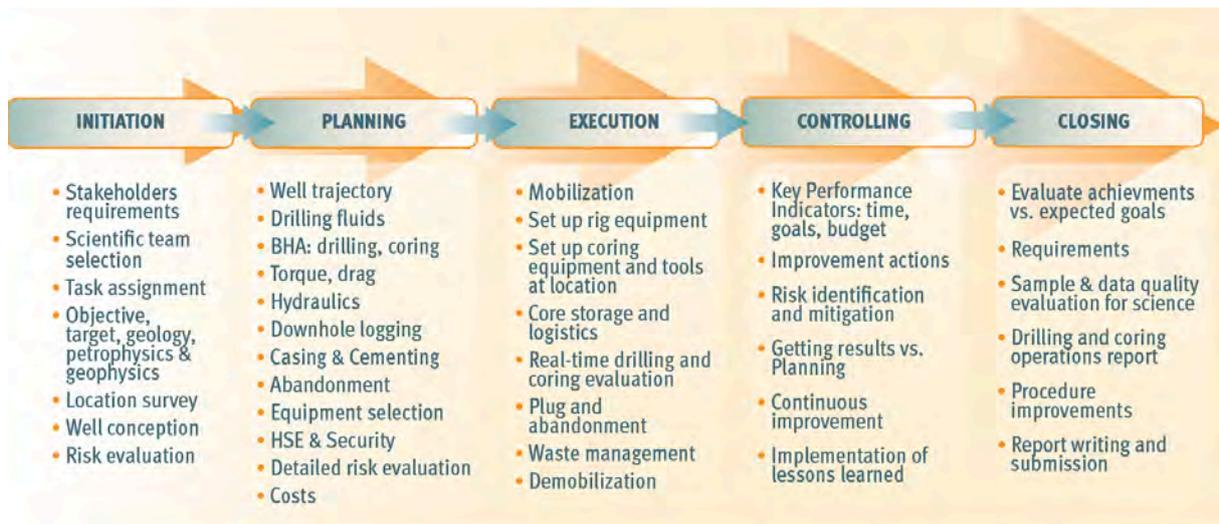
Fig. 4.2.6: Planning phases and well life cycle
