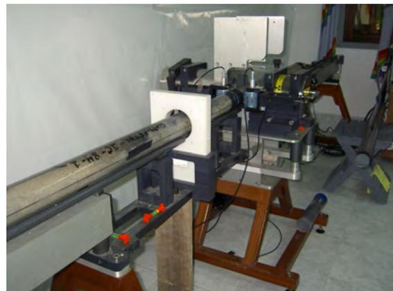
Fig. 5.9: Multisensor core logger in field lab
