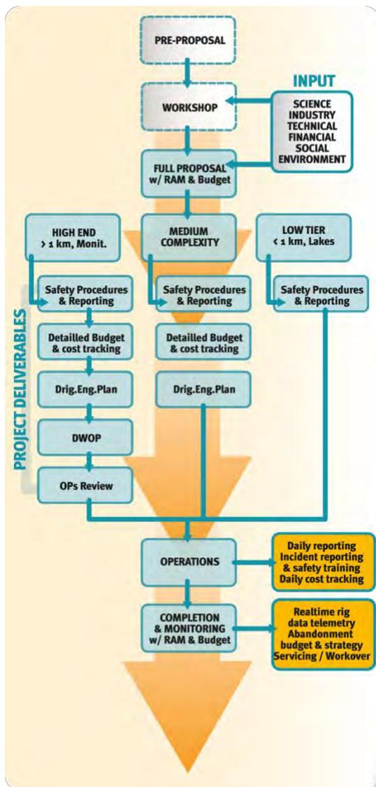
Fig. 3.7.2: Risk management for ICDP projects; see text for detailed description. (RAM: risk assessment matrix; DWOP: drilling well on paper); Ops review: post drilling operational review)
