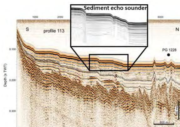
Fig. 4.1.11: Comparison of airgun seismic and sediment echo sounder data. Note the different resolution and penetration. The data have been collected with the system shown in Fig. 4.1.10.
