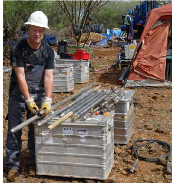
Fig. 4.6.15: OSG slimhole wireline logging sondes at a drill site
