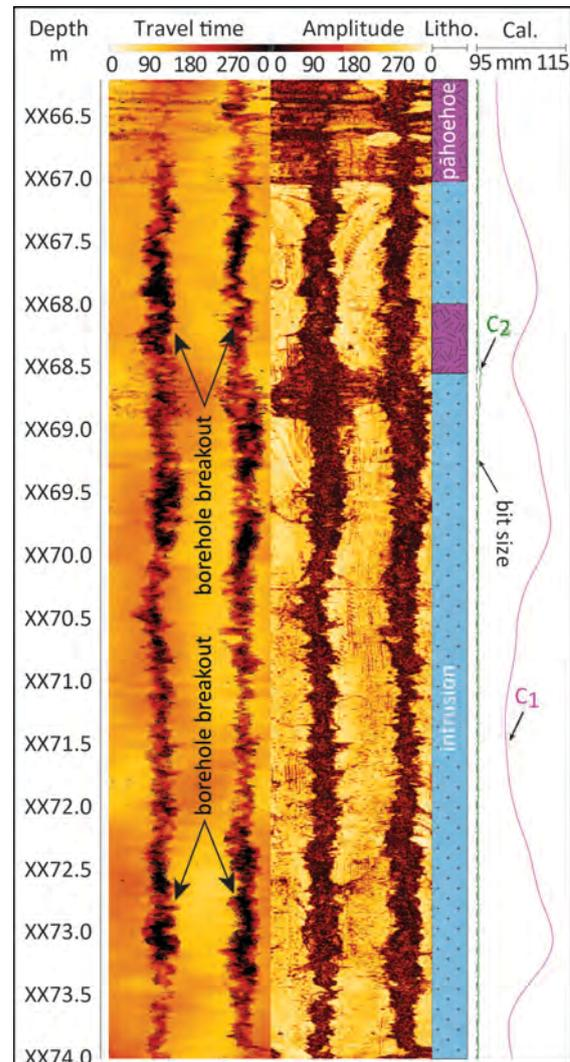
Fig. 4.6.11: Borehole breakouts appear as pair of dark, patchy stripes on opposing sides of the wellbore wall characterized by low amplitude and high travel time values.
