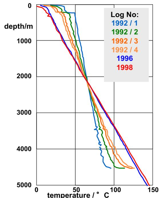
Fig. 4.6.6: An example of temperature equilibration in a deep borehole. The curves from 1992 were measured after the hole was drilled to 4500 m.
