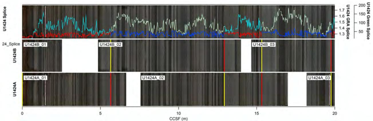
Fig. 4.5.16: Spliced line-scan images produced on cores from Hole-A -and- B during IODP Exp 346 overlaid by corresponding physical property data (GRAPE and RGB) for the top 20 mbsf. Note that both images and data from corresponding holes are computed into a scaled composite profile based on splice and offset (i.e. 'affine') tables, which are an essential output produced with the CORELYZER and CORRELATOR applications.
