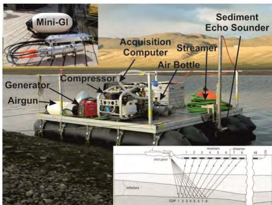
Fig. 4.1.10: Setup of an airgun reflection seismic system consisting of a Micro-GI Gun (modified Mini-GI Gun), a single mobile diving compressor, an air bottle for intermediate storage of compressed air, a 50-long 32 channel digital streamer and an acquisition system; upper left: image of a Mini-GI gun; lower right: principle of seismic reflection profiling.
