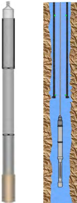
Fig. 4.6.2: Sketch of a sonde combination comprising total gamma ray, spectrum gamma ray and magnetic susceptibility, from top to bottom (left). A logging sonde is run through a coring drill string and the bit after the inner core barrel has been pulled out (right).
