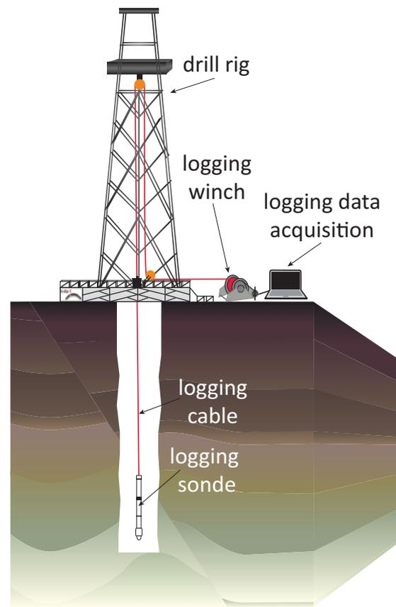
Fig. 4.6.1: Downhole logging scheme.
