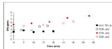
Figure 5-4 Methane concentrations over time in an opaque ("dark") chamber.
