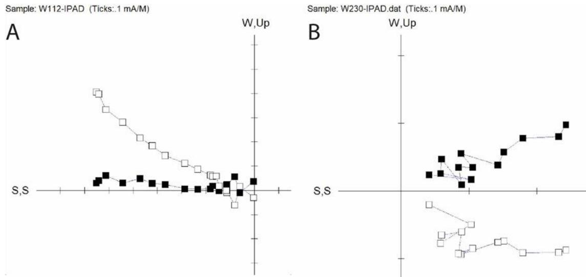
Figure 3. Orthogonal vector diagrams illustrating the alternating field (AF) demagnetization of two samples from the Sinemurian and Hettangian of the Wilkesley core. The closed and open symbols are projections onto horizontal and vertical planes, respectively; open symbols indicate polarity in this case. The sample in panel A (112' depth, mid *Bucklandi* Chronozone) is reversed polarity and the sample in panel B (230' depth, mid *Angulata* Chronozone) normal.
