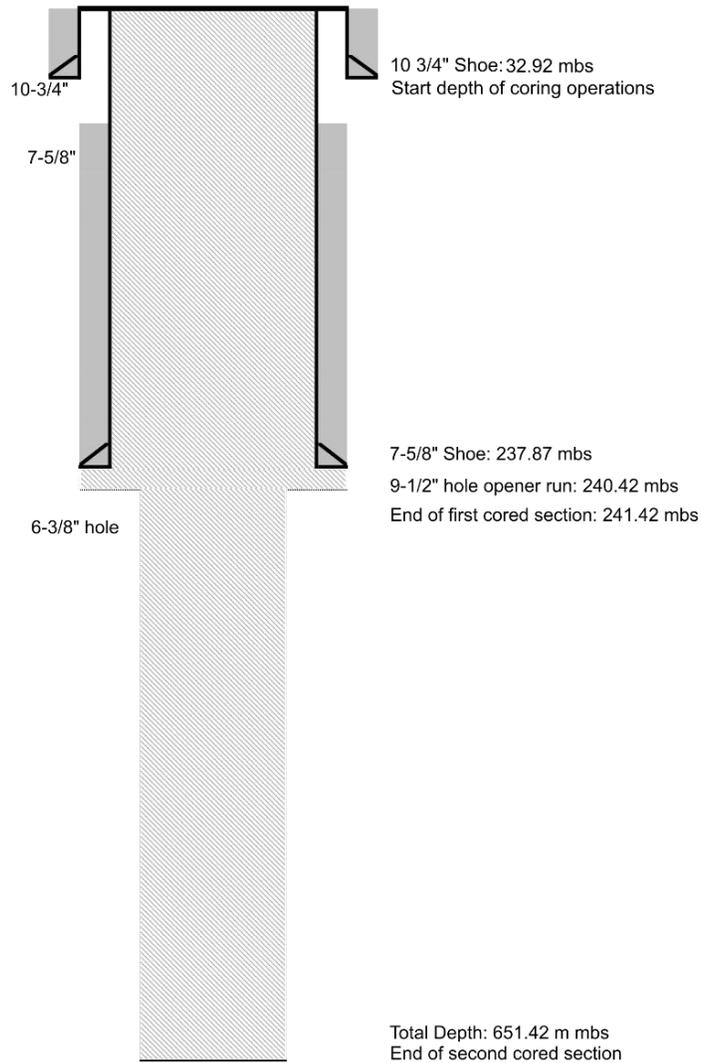
Figure 7. 5065\_1\_C (Prees-2C) well schematic illustrating the casing points and final borehole diameter after the completion of drilling operations (courtesy of Marriott Drilling Group).
