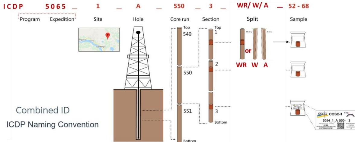
Figure A1. Example for the naming convention used in ICDP. The combined\_id is used in ICDP to name any site, hole and drilled or cored material. The ICDP expedition code for the JET project is 5065 (altered after Harms, 2021).
