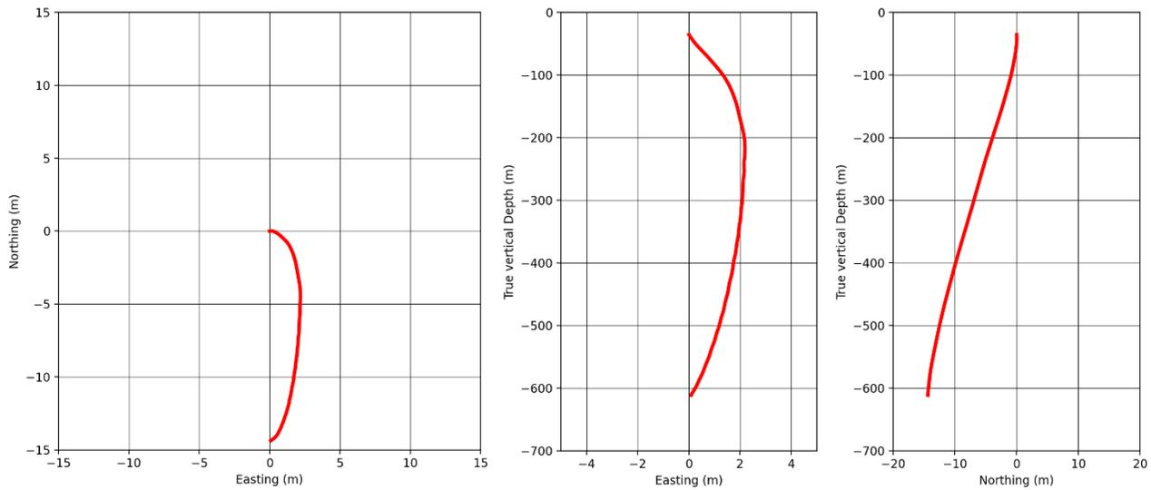
Figure 9. 5065\_1\_C borehole deviation survey. Trajectories calculated using the minimum curvature method.
