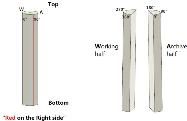
Figure 10. ICDP core marking conventions used during the JET geoscientific drilling to indicate the core top and working (W) and archive(A) halves (Harms, 2021).
