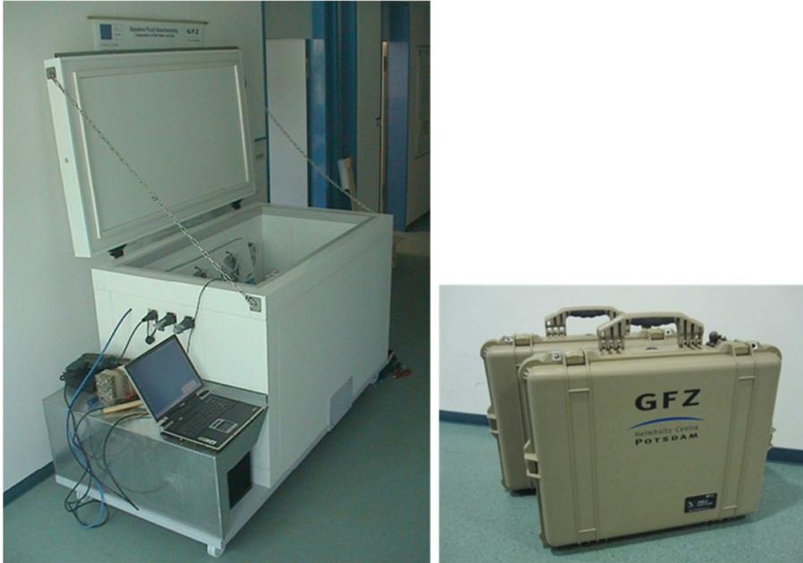
**Figure 2:** Edgewise and top view of the first set-up of the DAFGAS analytical unit. Main components inside the water vapour tight and air conditioned box are the mass spectrometer with a PC, a pump and a data logger. For details see the technical annex, section A 1.1.
