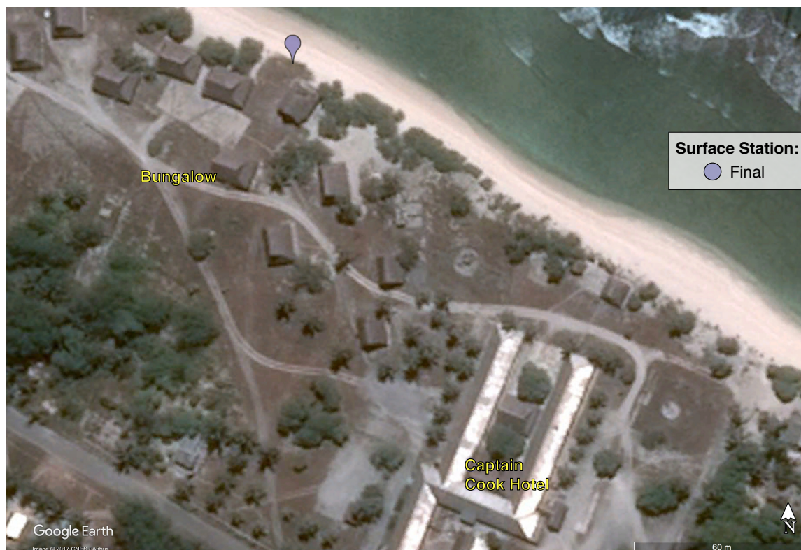
Figure 2: Aerial view of the Captain Cook Hotel property on Kiritimati Island, including the CXENRR site (upper left). The final location of the surface meteorology instruments is at the base of the pin symbol, north-northeast of the bungalow that housed staff and the Vaisala DigiCORA sounding system. The concrete pad where the helium tanks were stored and from which balloons were launched runs northwest to southeast, ending just north of the bungalow. The main hotel building used for internet access is southeast of the CXENRR site.
