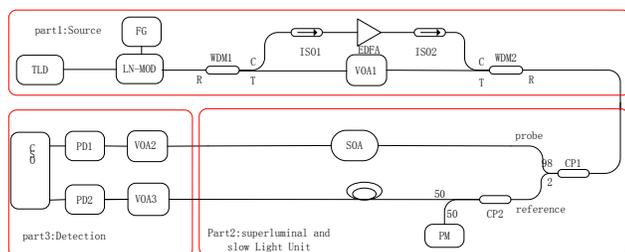
Fig. 5. Experimental setup to check the effect of superluminal and slow light in SOA. TLD, tunable laser diode; PD, photo-detector.
