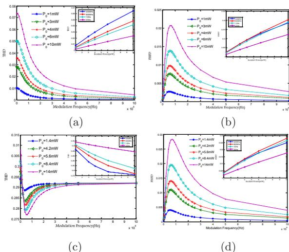
**Fig. 2.** THD and FHFD as a function of the modulation frequency and the incident power: (a) THD of sinusoidal signal, (b) FHFD of sinusoidal signal, (c) THD of rectangle signal, and (d) FHFD of rectangle signal.
