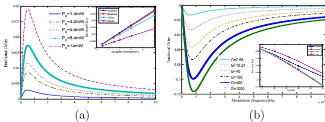
Fig. 1. Fractional delay with a sinusoidal modulated signal injected into SOA, while the incident powers are 1.4, 4.2, 5.6, 8.4, and 14 mW (a) without injection and (b) with different injection currents (different gain) for a particular incident power of 1 mW. The insets show FHF D of signal at different modulation frequencies 400 and 800 MHz, 1 and 2 GHz with different incident powers.
