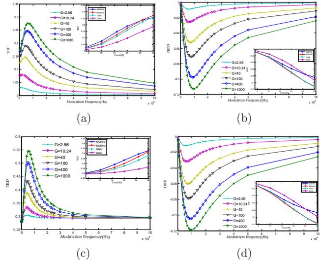
**Fig. 3.** THD and FHFD as a function of the optical gain in the SOA for the sinusoidal and rectangle waveform signals: (a) THD of sinusoidal signal, (b) FHFD of sinusoidal signal, (c) THD of rectangle signal, and (d) FHFD of rectangle signal.
