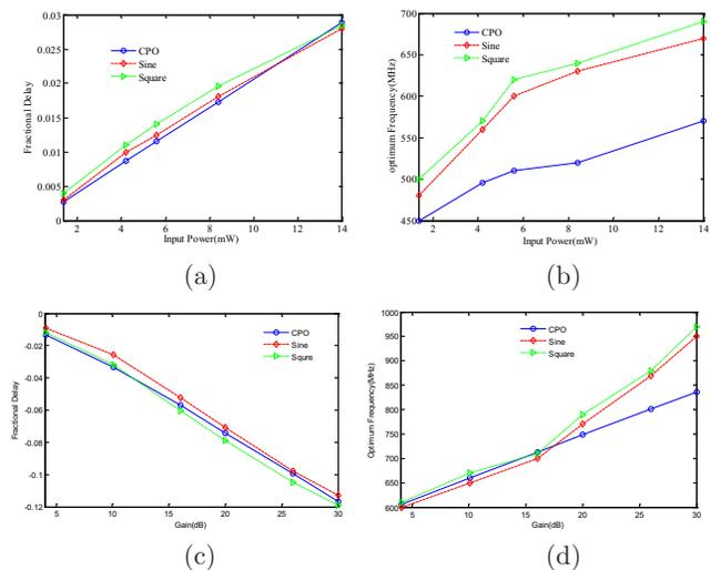
**Fig. 4.** Dependence of the maximum fractional delay and its corresponding modulation frequency: (a) and (b) show the dependences on the incident power; (c) and (d) show the dependences on the gain.
