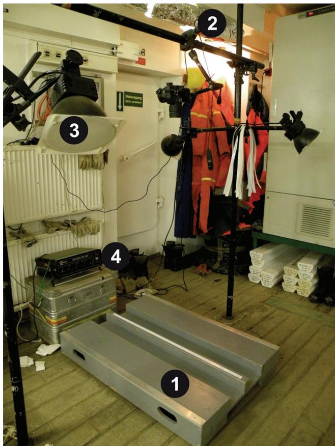
*Fig. 21: On-board photography system. Numbers label the different parts where particular attention is required. 1 the support orientation. 2 the room light intensity. 3 spot orientation. 4 spot light intensity control.*
