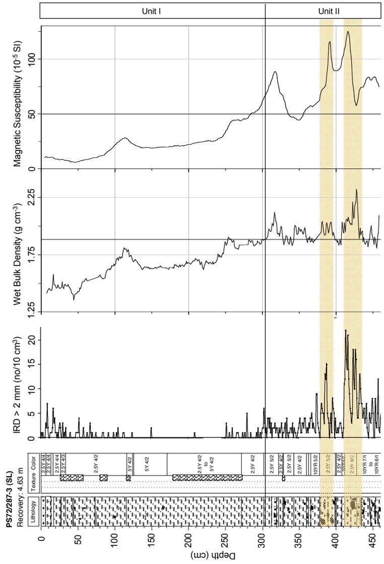
Fig. 34: Lithology, amount of IRD >2 mm (counting in X-Ray photographs), and wet bulk density and magnetic susceptibility from multi-sensor core logging of Core PS72/287-2.
