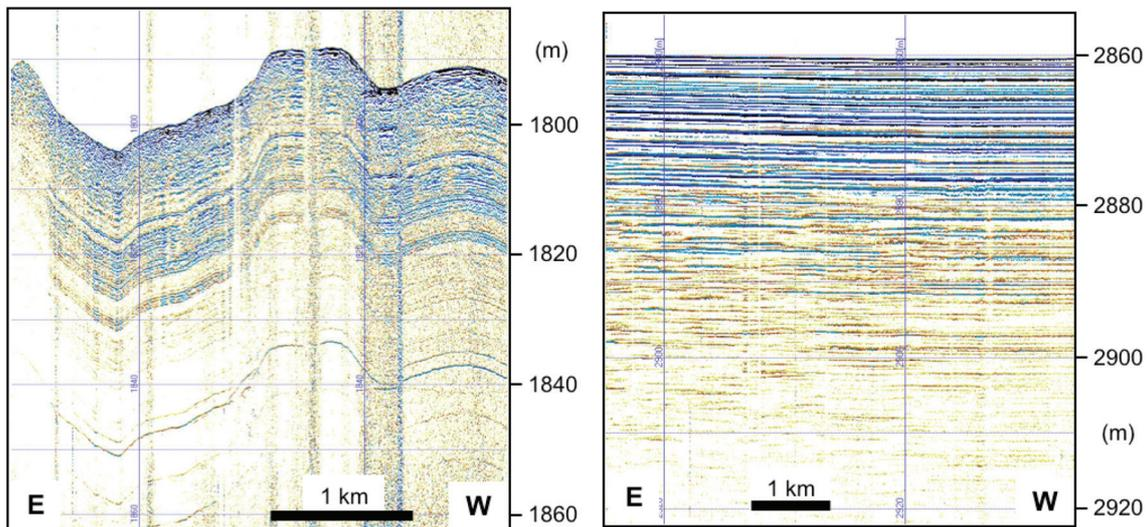
Fig. 11: Left: Parasound example from the top area of the Mendeleev Ridge. Coring location PS72/410 is at right end of the profile. Data processing: negative flank suppressed. Right: Parasound example from the Makarov Abyssal Plain. Coring location PS72/430 is at right end of the profile. Data processing: negative flank suppressed, two traces stacked to one.
