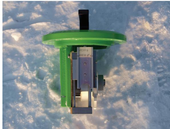
Fig. 66: 24 Hours Assembly with coated Sampling Slide
