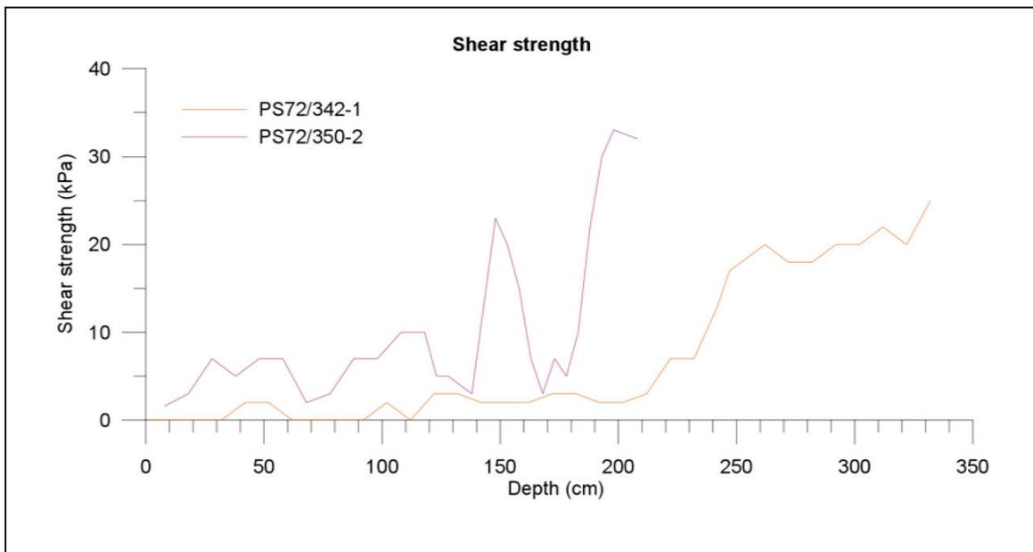
Fig. 15: Shear strength of core PS72/342-1 and PS72/350-2 from the Arctic Ocean. Both cores show a rapid increase in shear strength, caused by changes in lithology.
