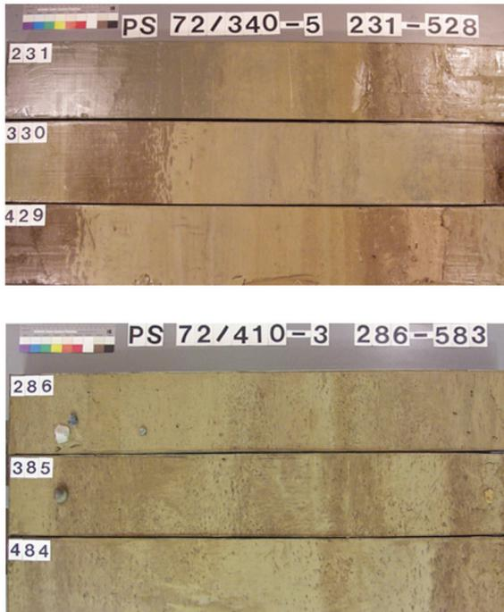
*Fig. 22: Two examples of pictures from KAL. The upper part shows a bad photo of the core PS72/340-5 231 to 528 cm and the lower part shows a good photo of the core PS72/410-3 286 to 583 cm.*
