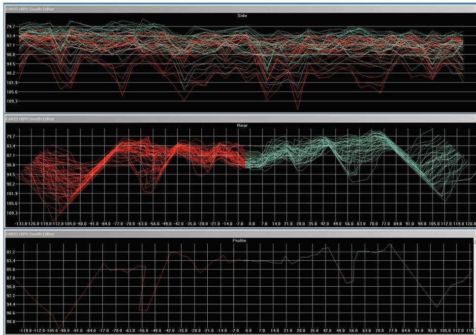
Fig. 62: Wrong depth measurements in shallow water
