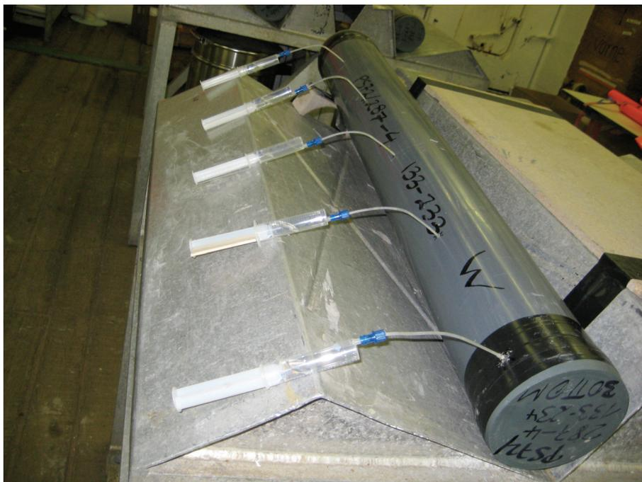
Fig. 42: Segments of Gravity Core sampled with rhizons and plastic syringes
