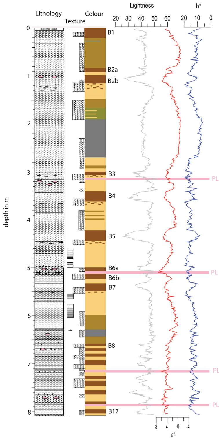
Fig. 13: Results of colour scanning and correlation with lithological core description sedimentary sequence of Core PS72/340-5
