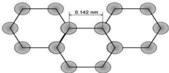
**Figure 3- Structure of graphene.**
