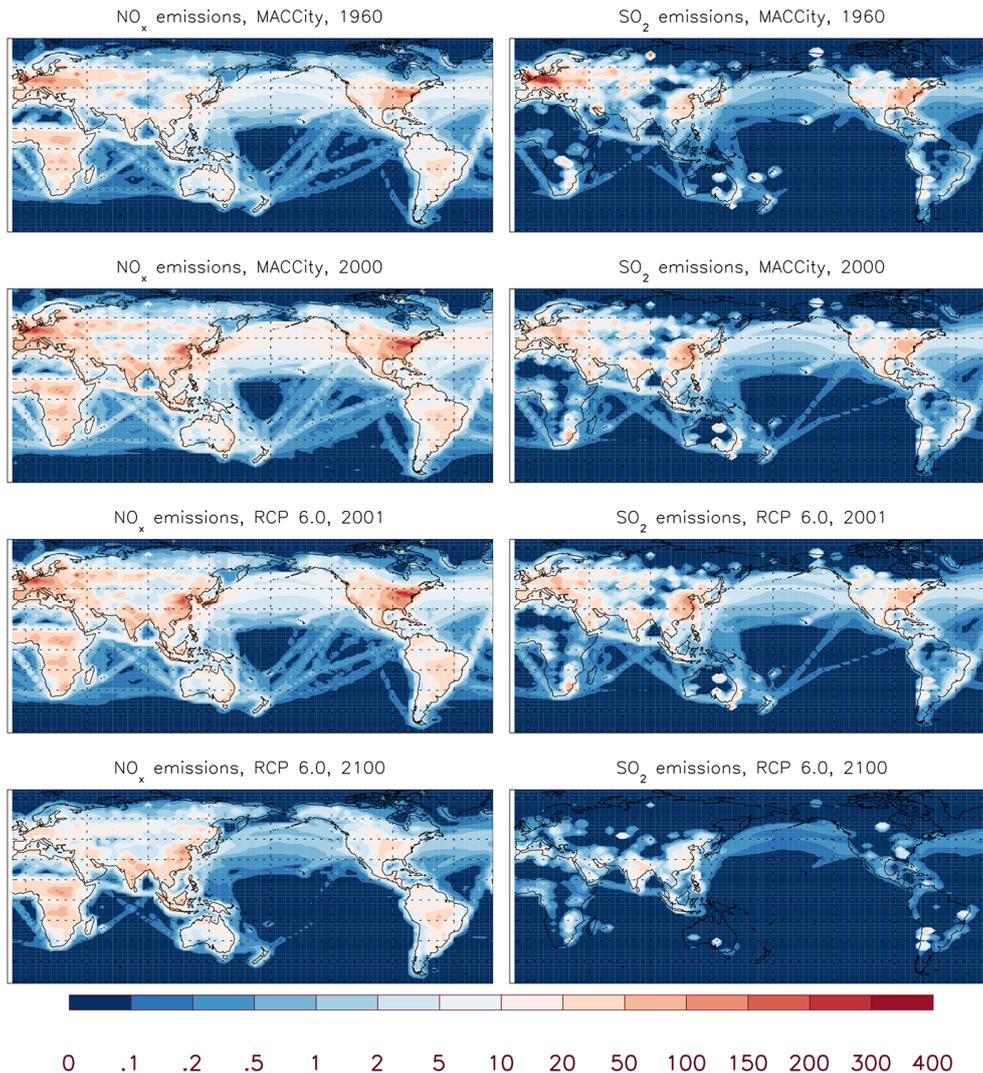
**Figure 2.** (left) Annual-mean  $\text{NO}_x$  surface emissions ( $10^{-12} \text{ kg (NO}_2\text{) m}^{-2} \text{ s}^{-1}$ ) in 1960 and 2000, taken from the MACCity emissions database, and in 2001 and 2100, taken from RCP 6.0. (right) Same, but for  $\text{SO}_2$  in ( $10^{-12} \text{ kg (S) m}^{-2} \text{ s}^{-1}$ ). Displayed here are the combined surface and stack-height emissions, excluding volcanic emissions.
