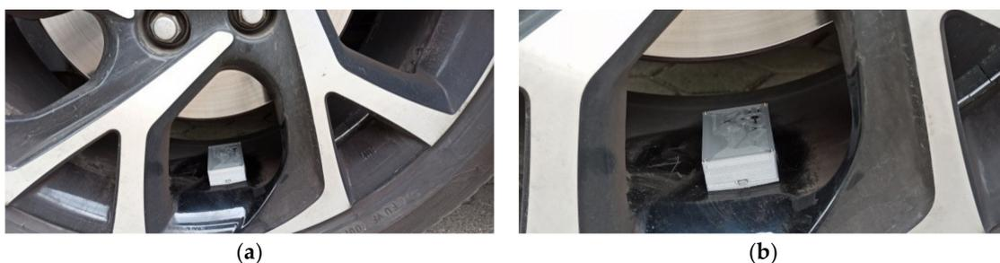
**Figure 5.** The head of wireless accelerometer (WA) view that is used in examinations: (a) Distant view; (b) Close view.
