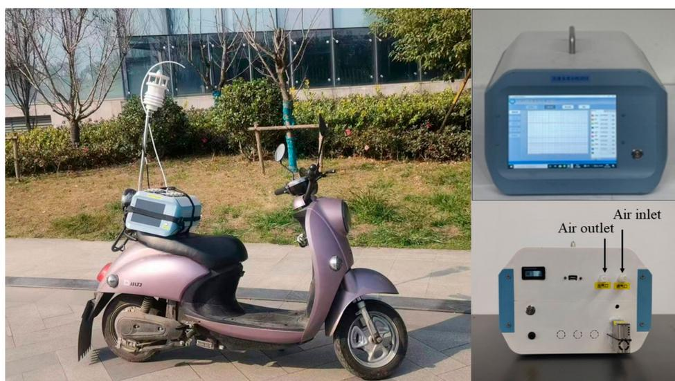
**Figure 3.** The sensor package fixed position on the bicycle (**left panel**) and the air inlet position of the sensor package (**right panels**).
