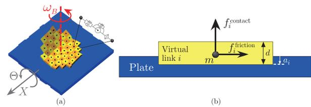
**Fig. 2.** Dynamic nonprehensile manipulation for rotating a deformable object using a plate with two degrees of freedom. Simulation model in (a) and the contact model in (b).
