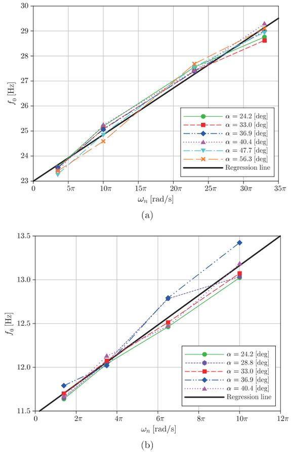
**Fig. 10.** Relationship between the object’s first order natural angular frequency in bending  $\omega_n$  and the parameter  $f_0$  obtained from the nonlinear regression of  $f_p$  vs.  $\omega_B$ , for (a)  $A_p = 3^\circ$  and (b)  $A_p = 12^\circ$ , with  $B_p = 3$  mm.
