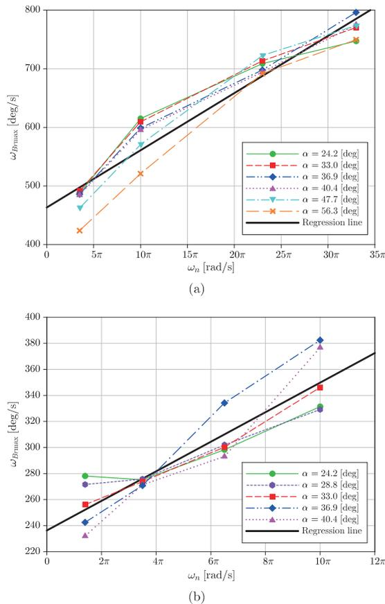
**Fig. 9.** Relationship between the object’s first order natural angular frequency in bending  $\omega_n$  and the parameter  $\omega_{Brmax}$  obtained from the nonlinear regression of  $f_p$  vs.  $\omega_B$ , for (a)  $A_p = 3^\circ$  and (b)  $A_p = 12^\circ$ , with  $B_p = 3$  mm.
