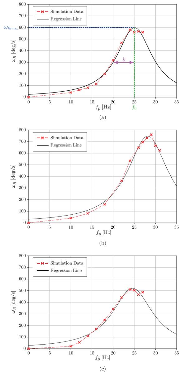
**Fig. 7.** Relationship between the object's angular velocity  $\omega_B$  and the plate's frequency  $f_p$ , for (a)  $\omega_n = 10\pi$  rad/s,  $\alpha = 36.9^\circ$ , (b)  $\omega_n = 33\pi$  rad/s,  $\alpha = 36.9^\circ$ , and (c)  $\omega_n = 10\pi$  rad/s,  $\alpha = 56.3^\circ$ .
