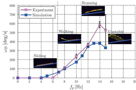
**Fig. 4.** Simulation and experimental results. The object's behavior changes similar to sliding, walking and running gaits [17].
