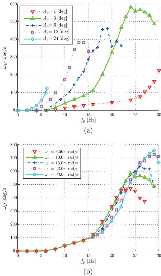
**Fig. 5.** Relationship between the object’s angular velocity  $\omega_B$  and the plate’s motion frequency  $f_p$  with respect to (a) the plate’s angular amplitude  $A_p$  for  $\omega_n = 10\pi$  rad/s, and (b) the object’s first order natural frequency in bending  $\omega_n$  for  $A_p = 3^\circ$ . Both (a) and (b) with  $B_p = 3$  mm and  $\alpha = 36.9^\circ$ .
