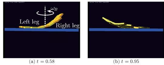
**Fig. 3.** Snapshots of the simulation for  $f_p = 12$  Hz,  $A_p = 12^\circ$ ,  $\omega_n = 10\pi$  rad/s and  $\alpha = 36.9^\circ$ . The object is rotating on the plate with an angular velocity of  $\omega_B = 344^\circ/\text{s}$ , by using a bipedal-gaited motion.
