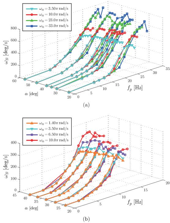
**Fig. 8.** Relationship between the object’s angular velocity  $\omega_B$  and the plate’s motion frequency  $f_p$ , for different friction angles  $\alpha$  and different deformable objects for (a)  $A_p = 3^\circ$  and (b)  $A_p = 12^\circ$ , with  $B_p = 3$  mm.
