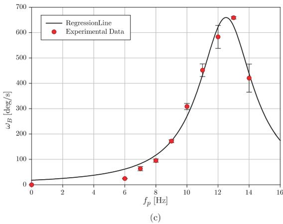
**Fig. 12.** Relationship between the object's angular velocity  $\omega_B$  and the plate's frequency  $f_p$ , for (a) a slice of cheese, (b) the skin of a Chinese dumpling and (c) a slice of cheese with lead balls, with  $A_p = 12^\circ$  and  $B_p = 3$  mm.
