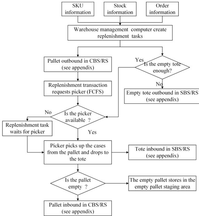
FIGURE 2. Flowchart of the replenishment transaction in the CAWS.
