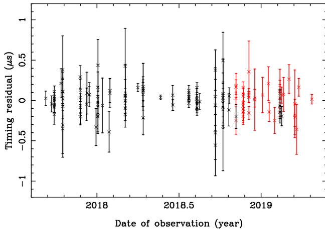
**Figure 5.** Timing residuals from PSR J1909–3744 obtained by the PPTA project team. Points in black are from observations with the 10-cm receiver and PDFB4 signal processor. Those in red are observations covering the same band, but with the UWL system.
