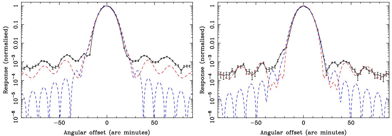
**Figure 8.** Beam pattern obtained through scans in azimuth (left) and elevation (right) for the 20-cm observing band (sub-band 5, Table 1). The measured response is shown using the black line and error bars. The red and blue dashed lines are modelled beam shapes that are described in the text.
