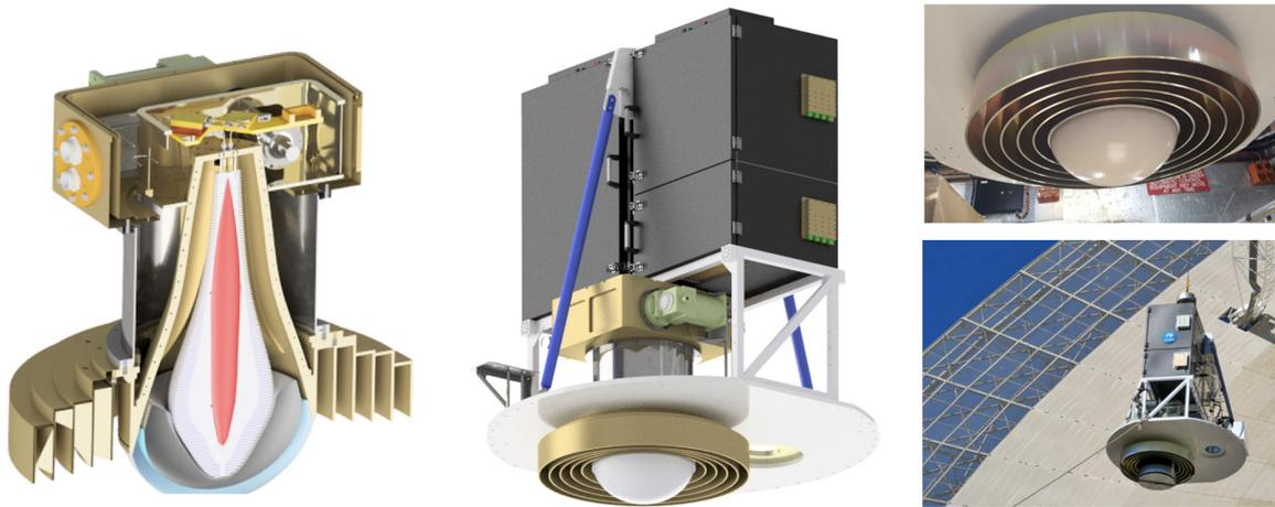
**Figure 2.** Representation of the feed system: (left) the internal structure of the feed, (centre) the feed, platform, and RF shielded cabinets, and (right) the completed system being installed on the telescope.
