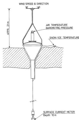
**Fig. 5.1:** Scheme of a drift buoy from Hoerber & Gube-Lehnhardt (1987)
