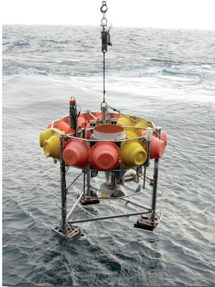
*Fig. 7.3: Long-term bottom-lander equipped with a current-meter, temperature and oxygen sensors, and a small sediment trap to collect settling particulate matter*
