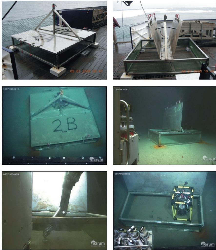
*Fig. 7.7: Cages of the starvation experiment on deck (top) and at the seafloor (middle); sediment sampling using push-corers (bottom, left) and measurements of dissolved oxygen in surface sediments inside the cages by means of an autonomous micro-profiler handled by the ROV*
