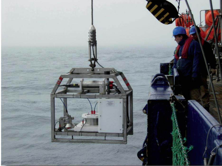
*Fig. 7.5: Deployment of the Ocean Floor Observation System (OFOS)*
