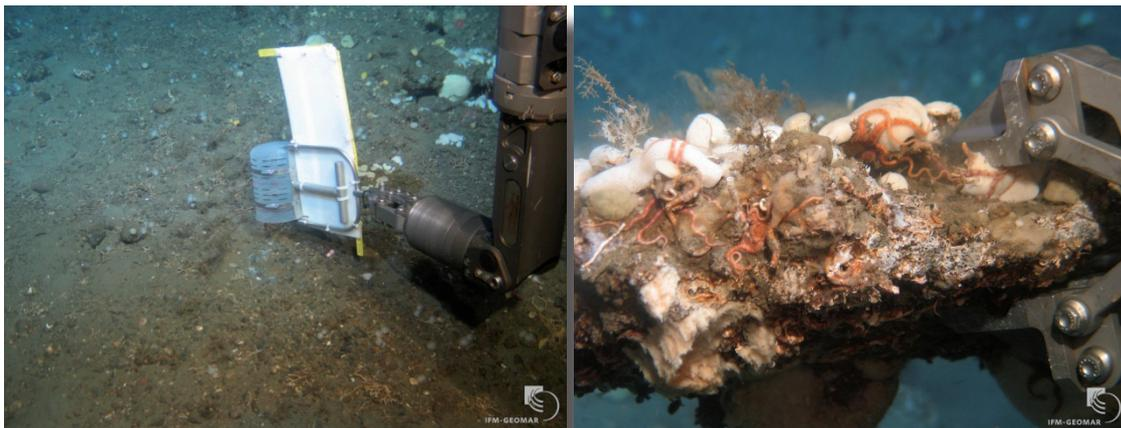
*Fig. 10.2: A perspex beaker is placed on top of a gas bubble hole (left). An autigenic carbonate sample densely populated by megafauna (right)*
