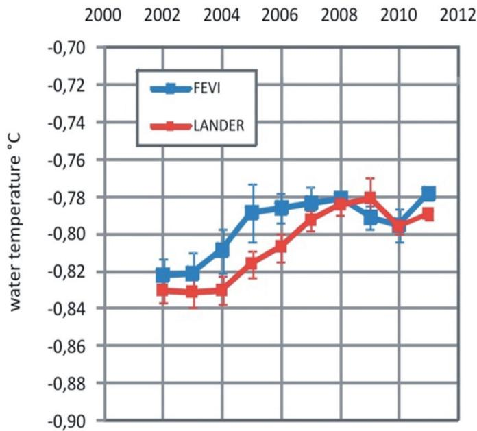
Fig. 7.10: Mean annual bottom-water temperatures at the central HAUSGARTEN site (2,500 m water depth) between 2002 and 2011; red line: 2.5 m (bottom-lander), blue line: 15 m (mooring) above the seafloor
