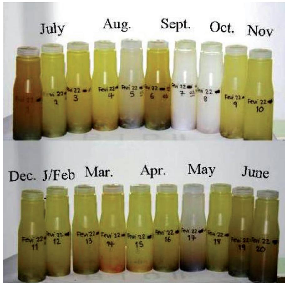
Fig. 5.1: Sampling jars of a sediment trap moored at the central HAUSGARTEN station in ~ 200 m depth obtained during 2010/11
