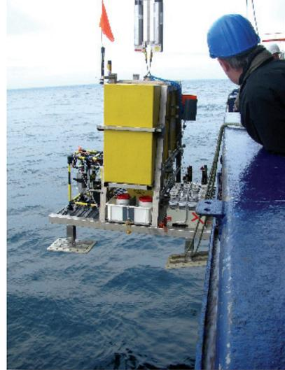
*Fig. 3.2: IFM-GEOMAR Ocean Elevator during launch, carrying microprofiler, “saltshakers”, pushcores and HOMER Beacons (Station 161ROV03)*
