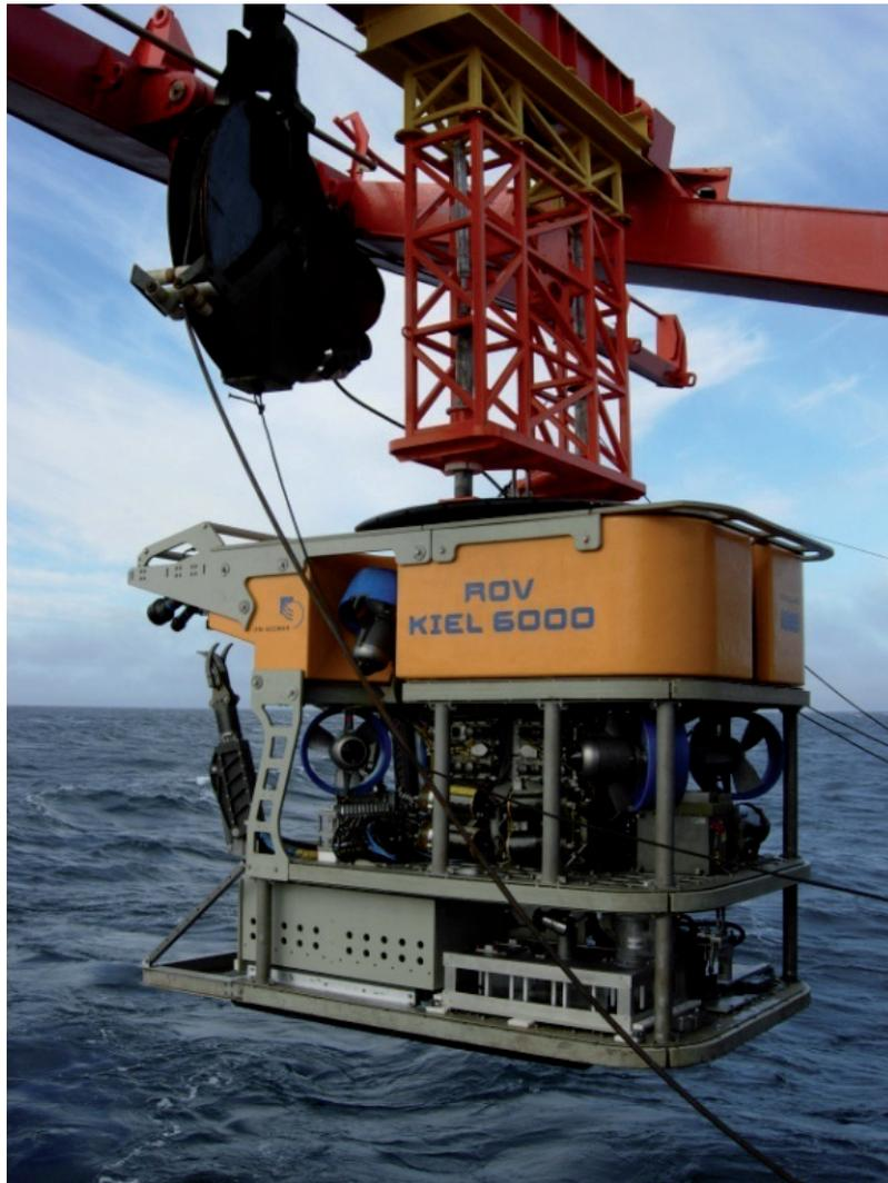
*Fig. 7.6: The ROV KIEL 6000 was used to collect surface sediments and benthic organisms, and to install and sample various biological long-term experiments at the deep seafloor*
