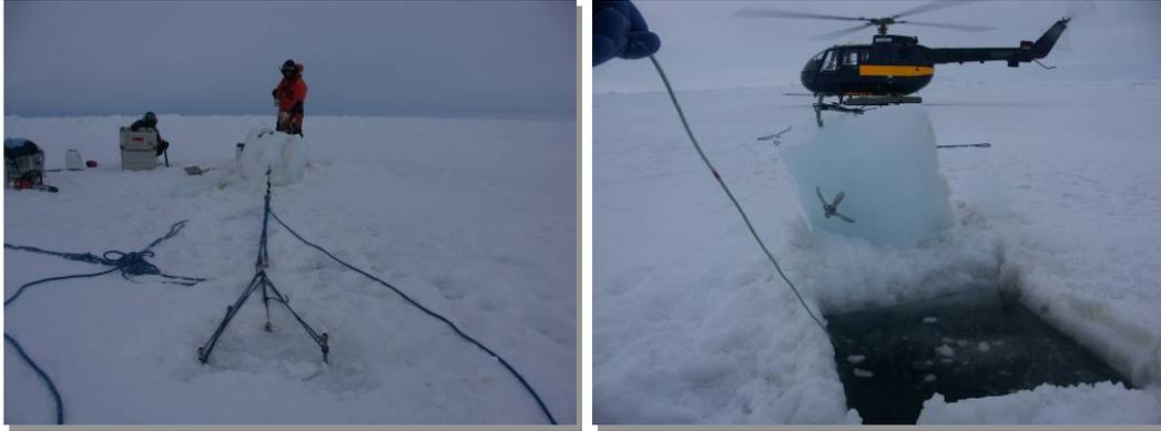
Fig. 17.1: The pulley system to prepare the sampling hole
