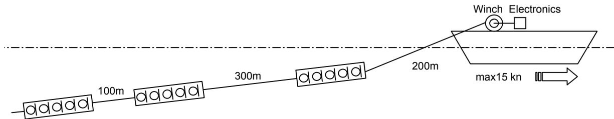
Fig. 16.1: Schematic drawing of the acoustic streamer
