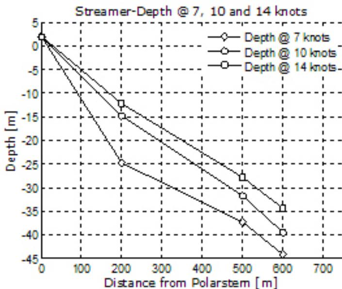
Fig. 16.2: Streamer depth as a function of tow speed. The markers at zero distance indicate the height of *Polarstern*'s working deck.
