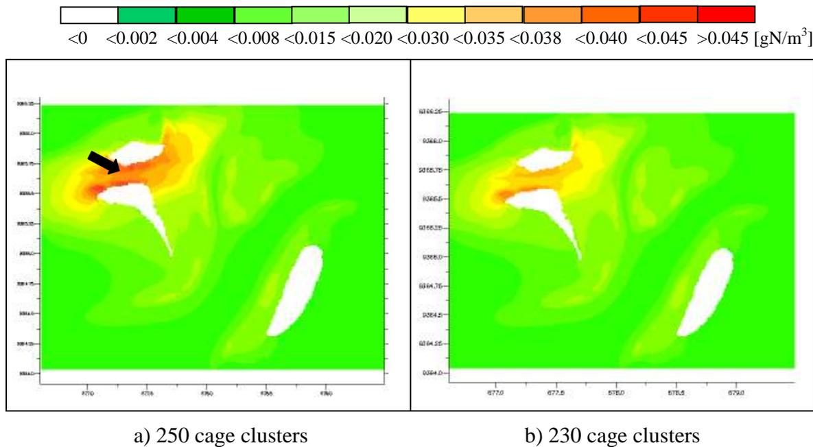
Fig. 10: Predicted  $NH_4$  concentrations for the proposed arrangement of the cage clusters.
