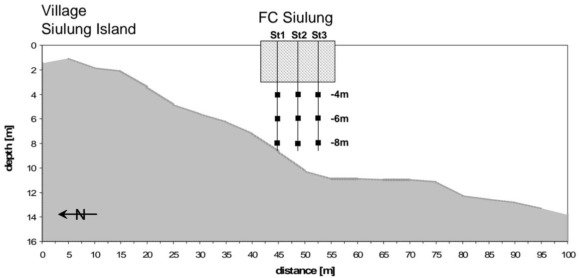
Figure 4: Sediment traps set-up below FC Siulung
