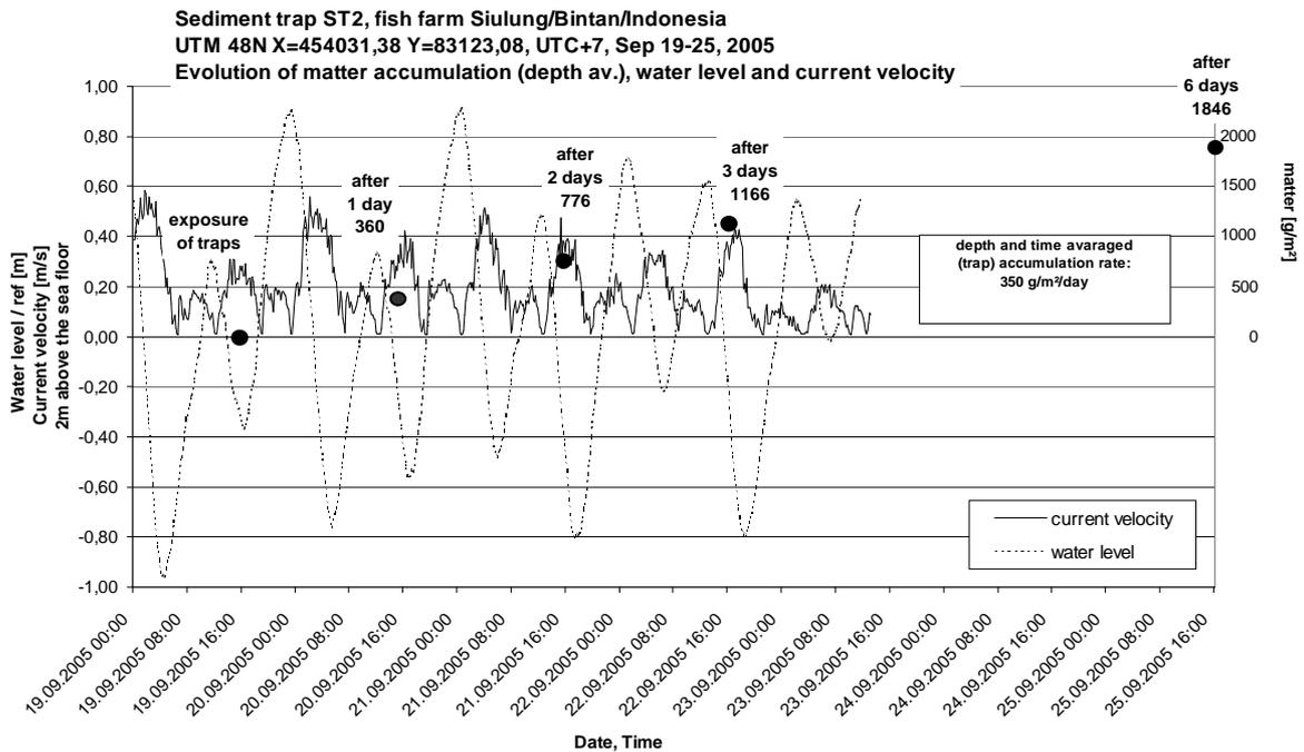
*Figure 8: Current velocity, water level and accumulation of matter*
