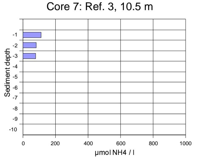
*Fig. 5 & 6: Vertical profiles of ammonia concentration in the porewater of reference stations 2 and 3*
