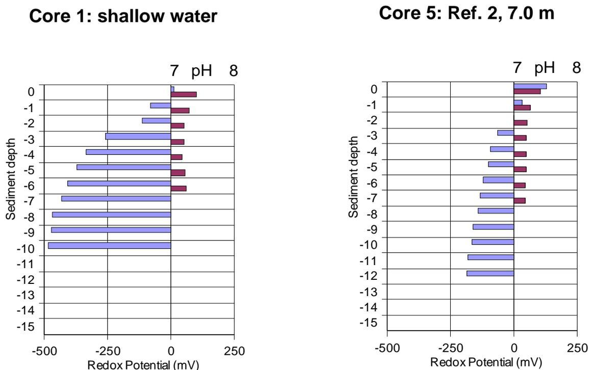
Fig. 2 & 3: Vertical profiles of redox potential (blue) and pH value (red) in sediments exposed to high organic input (Fig. 1, left) and lower organic input (Fig. 2, right)
