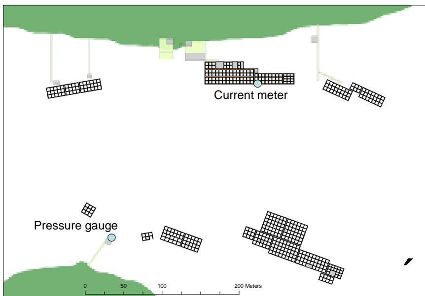
Figure 7: Propeller current meter and pressure gauge positions
