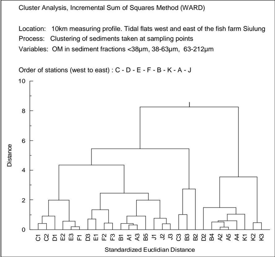
*Fig. 7 Grouping of sediments according to similarities of OM referring to the tested variables: grain size fractions  $<38\mu\text{m}$ ,  $38-63\mu\text{m}$  and  $63-212\mu\text{m}$  of sediments.*
