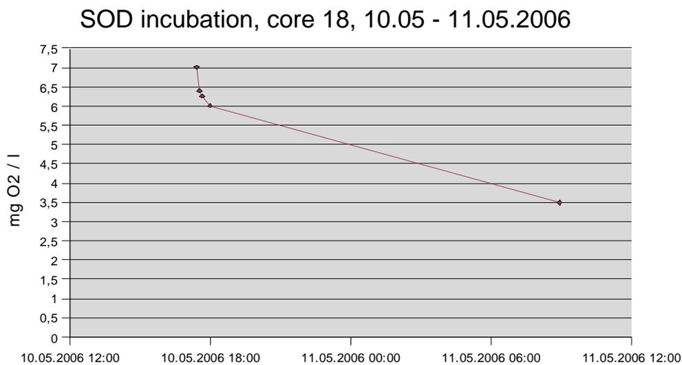
*Fig. 11: SOD incubation experiment: decrease of oxygen concentration in the overlaying water during 24 hours*
