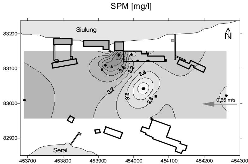
Fig. 4: Suspended matter dispersion between the islands of Siulung and Serai (average current speed in the channel indicated as arrow).
