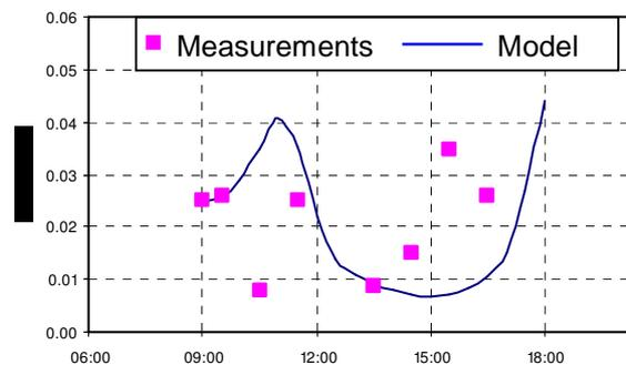
Fig. 6: Measured versus computed ammonium concentrations near the fish farm at Pramuka
