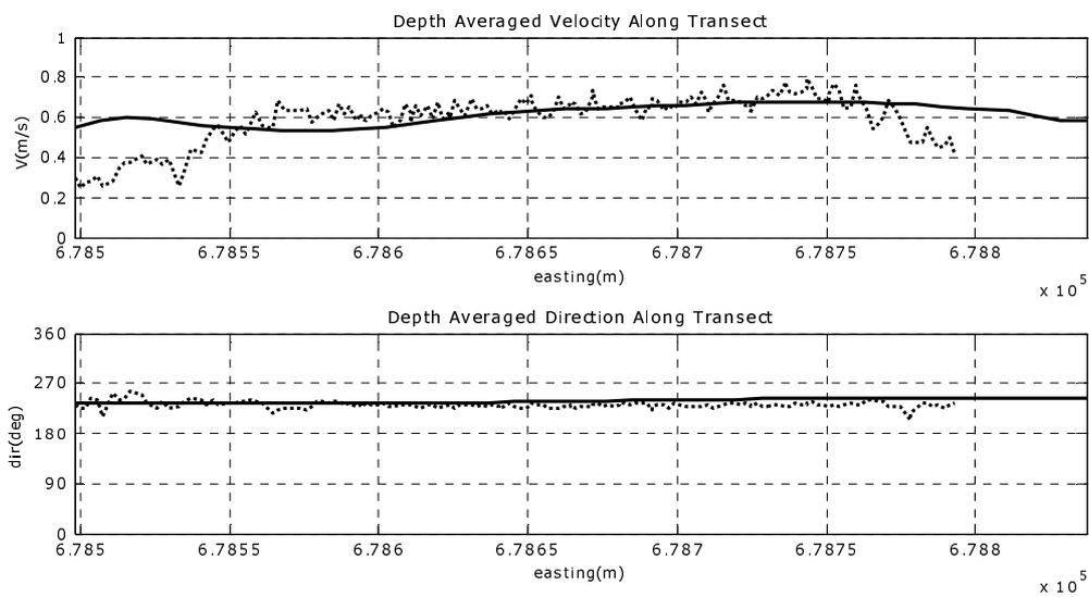
b) Magnitude and direction of current velocity over cross-section PT4
