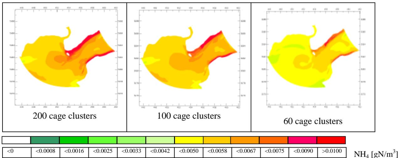
Figure 8. Determination of the site-specific holding capacity: Dissolved ammonium distribution for various number of fish farm cage clusters
