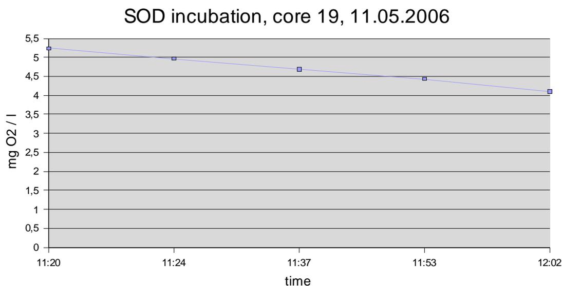
Fig. 12: SOD incubation experiment: decrease of oxygen concentration in the overlaying water during the first hour of experiment
