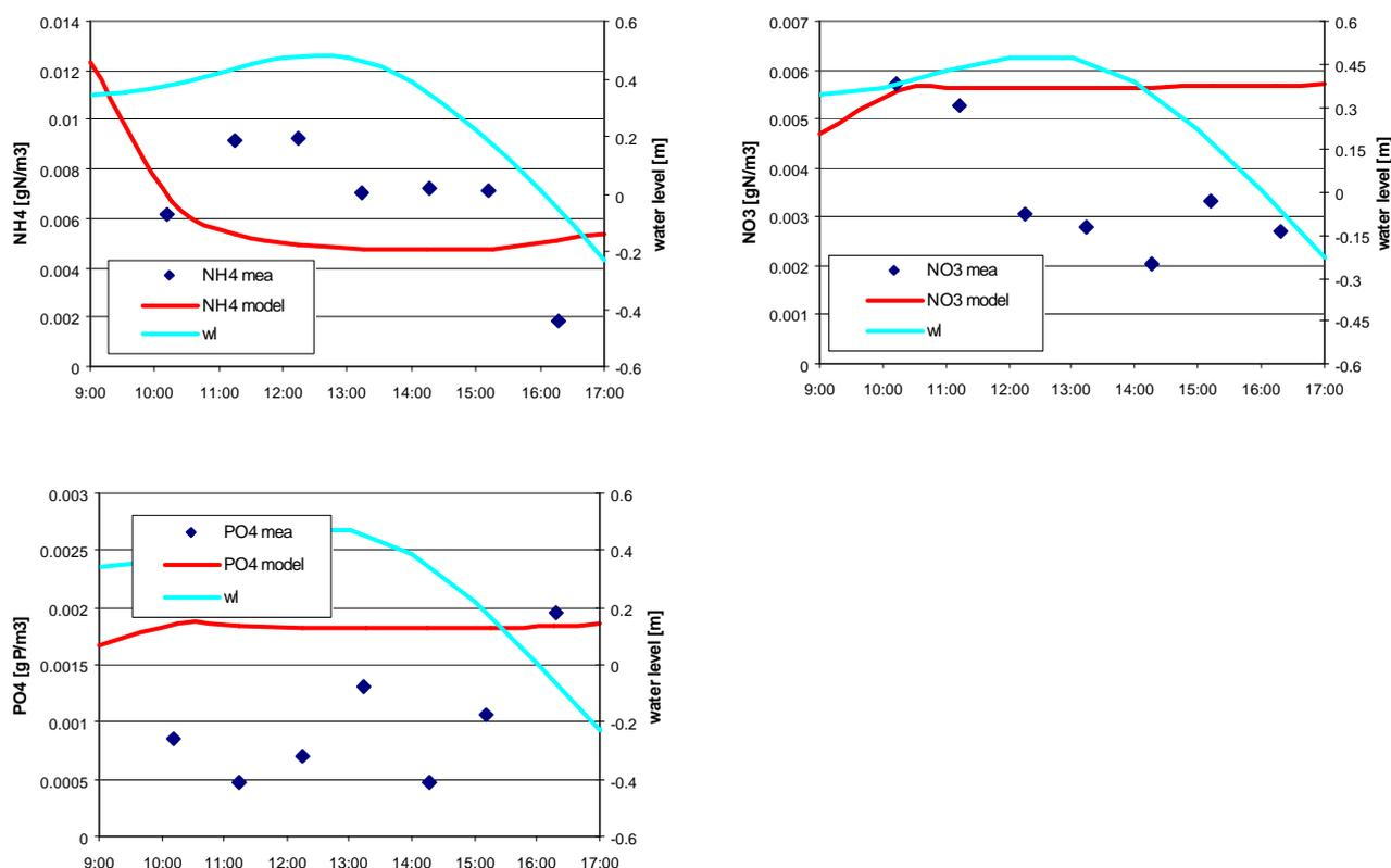
Figure 6. The measured vs. predicted nutrient concentrations after calibration in the vicinity of the fish farm.
