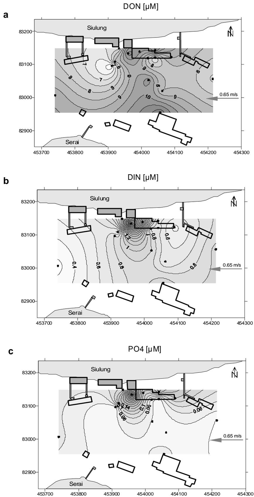
Fig. 3 a-c: Distribution of dissolved organic (a) and inorganic nitrogen (b) and phosphate (c) (cages indicated as transparent objects – cluster 2 is located in the centre close to Siulung).
