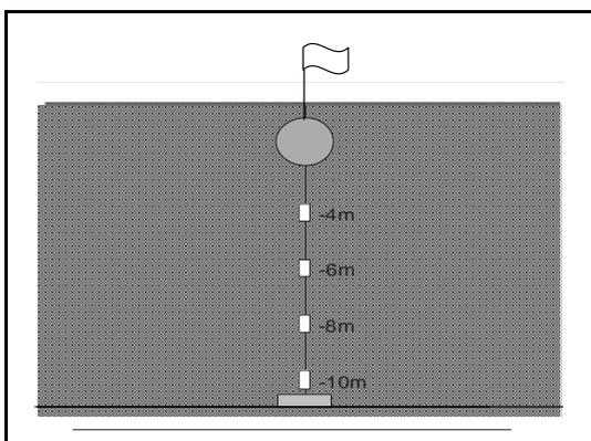
Figure 5: Design of the sediment trap sampling stations
