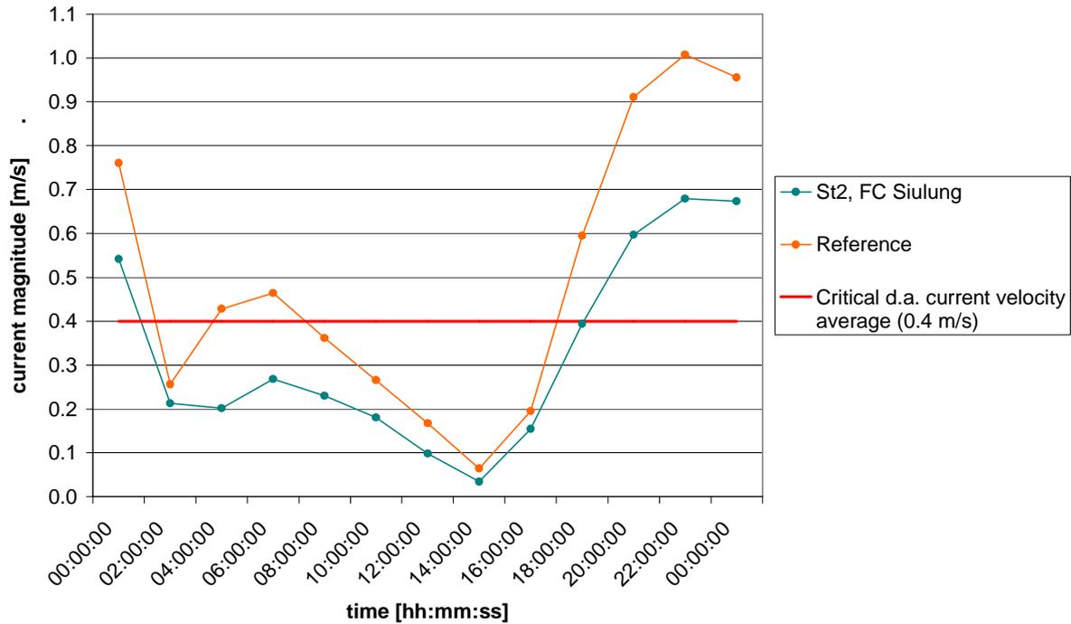
Figure 9: Current velocities at St2, FC Siulung (measured) and at REF2 (modelled). The dotted line indicates the critical current velocity (0.4m/s)
