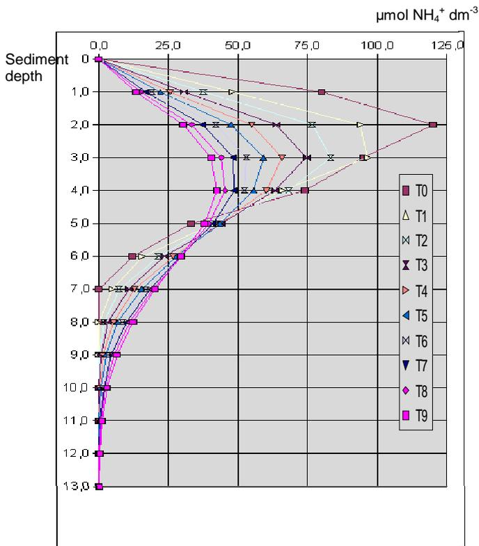
Figure 10 follows a (fictive)  $\text{NH}_4^+$  profile (T0) over 9 days (T1 – T9), using the same constants, assumptions and conditions as above. For each consecutive day, the new porewater concentrations were calculated according to Fick's first law. It becomes apparent, that the ammonia peak decreases while it moves from the initial depth of 2 cm down to 4 cm.
