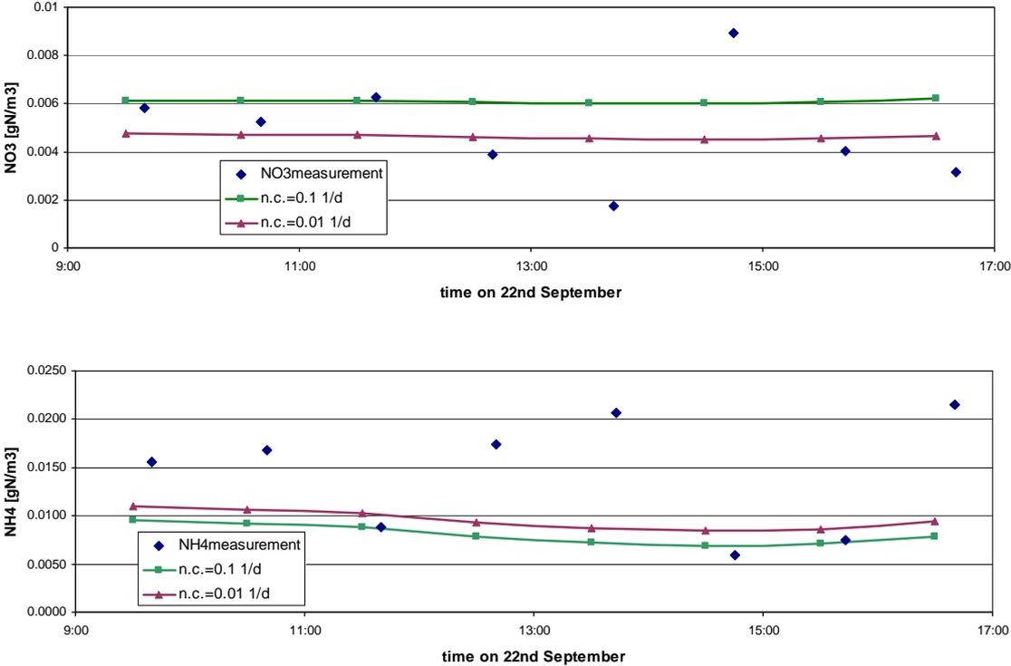
Figure 5. Measurement vs. model predictions of nutrient concentrations considering different first-order nitrification rates.
