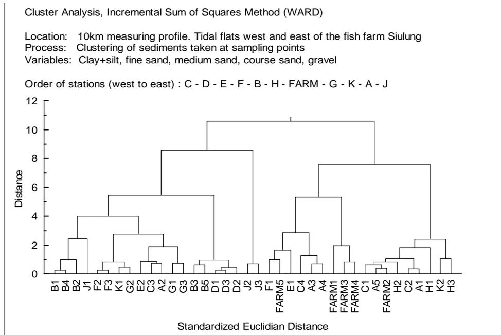
Fig. 5 Grouping of sediments according to similarities referring to the test variables.
