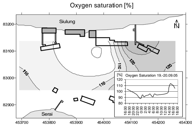
Fig. 7: Oxygen saturation between the islands of Siulung and Serai during daytime and diurnal variation at the fish farm (insert).
