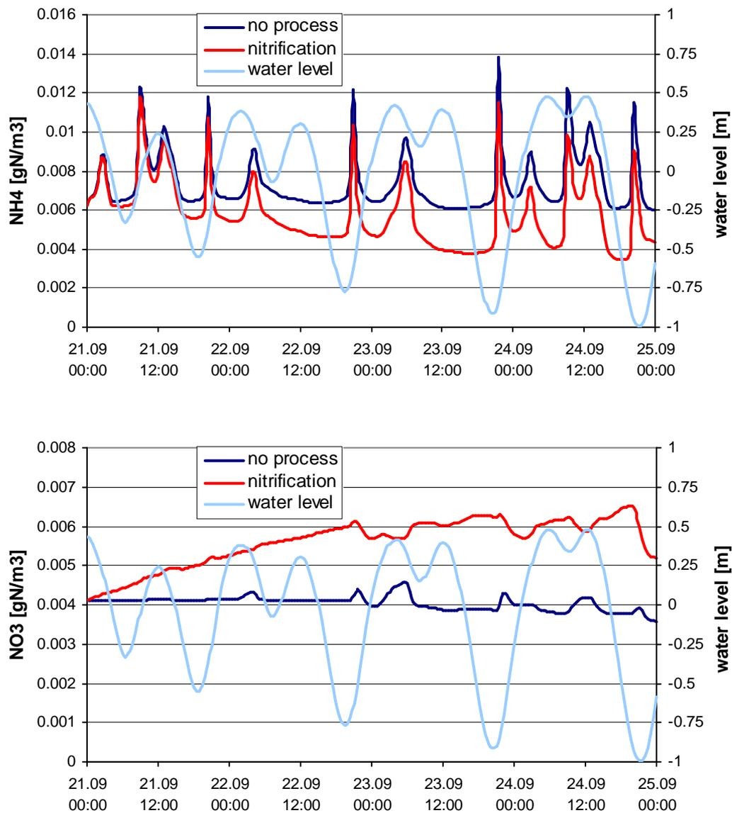
Figure 3. Effect of nitrification on ammonium and nitrate concentrations at the fish farm
