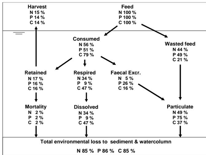
Figure 9: Feed distribution for N, P and C for the entire area, as an average of the entire modelled period.
