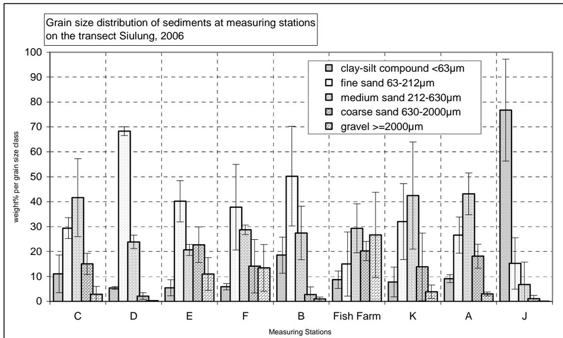
Fig. 4 Relative weightings of main grain size classes based on 3-5 sediment samples taken at each measuring station. The measuring stations are ordered according to their distance to the fish farm.
