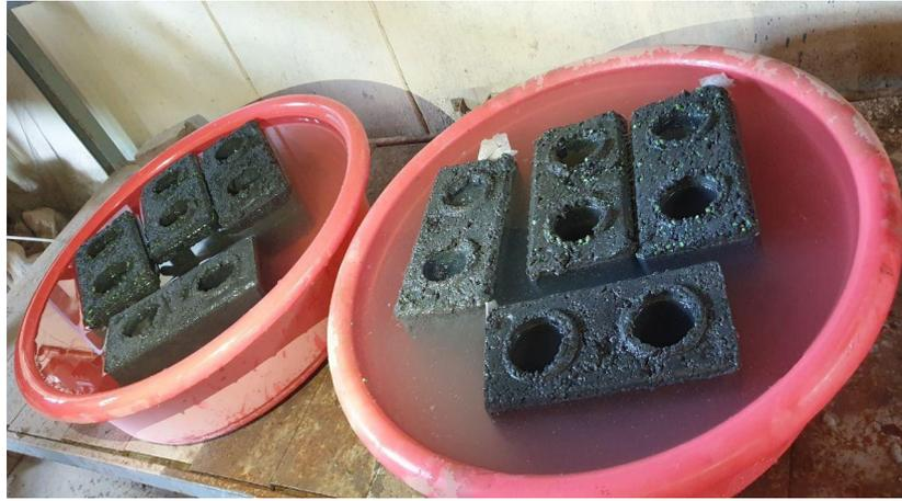
Figure 4. Plastic blocks in water dipping
