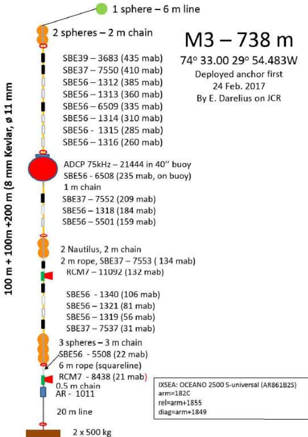
Figure 2: Drawing of mooring M3 (2017-2021)
