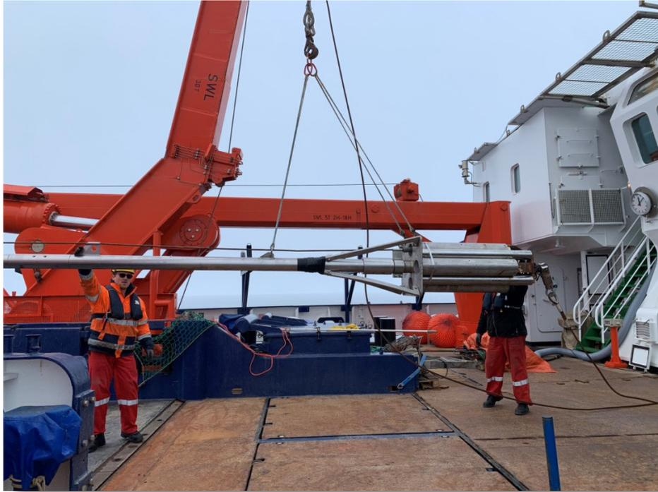
Fig. 6.1: Deployment of the 6 m heat flow probe was carried out over the stern. Very calm sea conditions made this a smooth operation. (Photo: J. Ritter)
