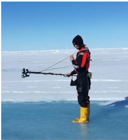
Fig. 11.2: Spectral measurement of the *Stickle* during melt pond transect in a small and shallow melt pond.
