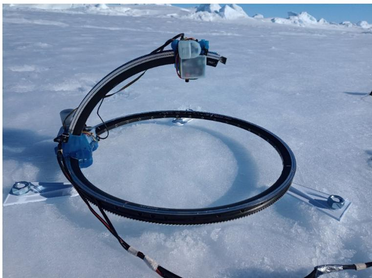
*Fig. 11.4: Goniometer position on 04 July 2023 with underlying thin ice layer on top of snow/ice surface*
