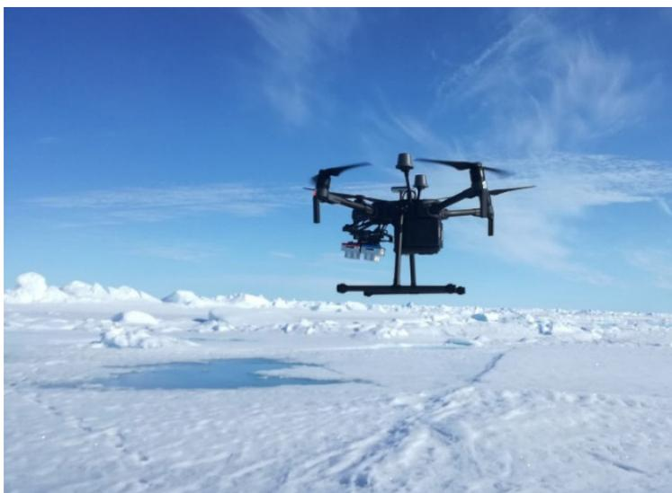
Fig. 11.1: DJI Matrice 210 RTK V2 with attached MicaSense RedEdge-MX Dual Camera.
