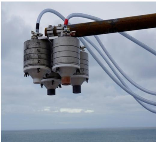
Fig. 7.1: Four filter pack systems collecting samples of  $\text{NH}_3$  and  $\text{NH}_4^+$
