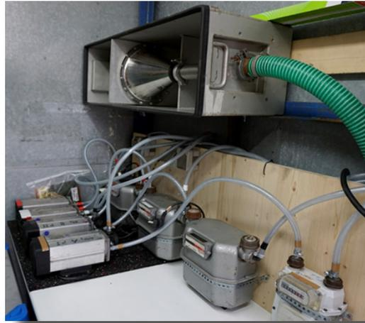
For the case of wind blowing from the tail a similar filter pack system was ready to be installed on the stern (Fig. 7.2). During PS102 it has not been necessary to use this extra system because the wind or relative wind came the most time from the front area.
