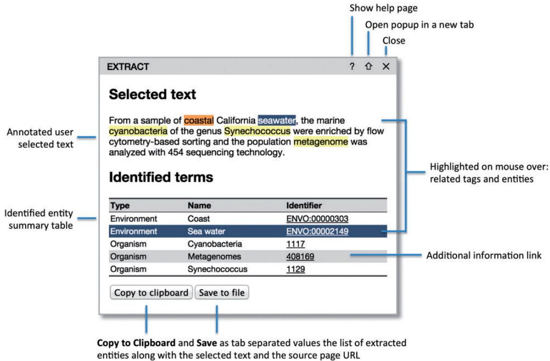
**Figure 1.** The EXTRACT popup. Hovering the mouse cursor over the text tags or the table rows enables users to visually inspect which words have been identified as which entities. To allow for easy collection of annotations in tabular form, e.g. in an Excel spreadsheet, two buttons allow the user to either copy the information to the clipboard or save it to a tab-delimited file. When doing so, the selected text and the address of the source web-page are also included for provenance.
