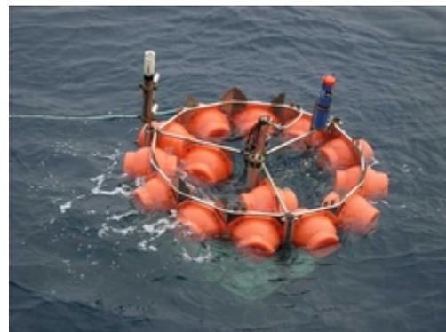
Upper ring of floats of a free-falling device (bottom-lander)(© T. Soltwedel, AWI)
