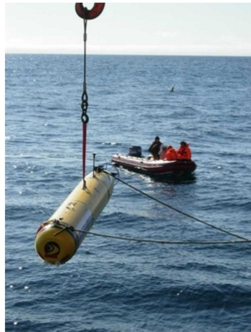
Deployment of the Autonomous Underwater Vehicle (AUV)(© T. Soltwedel, AWI)
