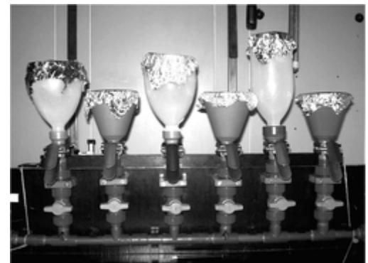
Rack allowing multiple filtrations of seawater samples
