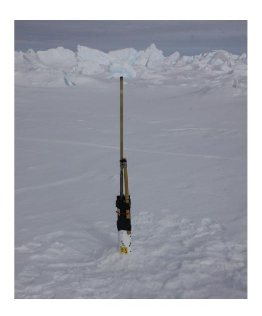
"Deformation Array" to study the motion and deformation of a distinct area.
