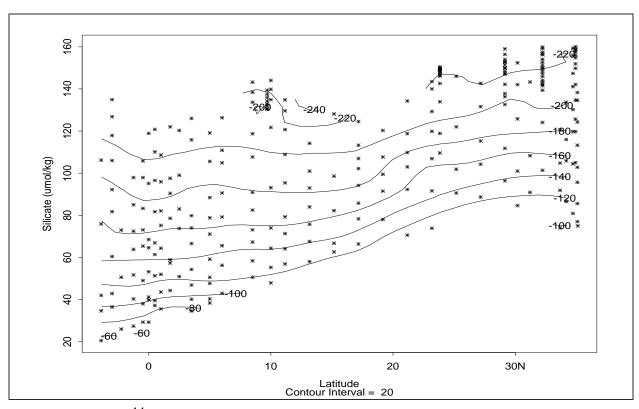
**Figure 4:** Section of <sup>14</sup>C contours along latitude in silicate space for the 500-2500m depth range. Note that for this section, "shallow" is toward the bottom.
