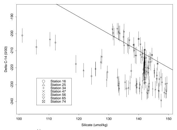
**Figure 6:** All LV  $\Delta^{14}$ C measurements having a quality control flag value of 2 or 6 are plotted. Vertical bars are one sigma errors. The heavy line is that suggested by Broecker, *et al.* (1995) to be representative of the global relationship between pre-bomb  $^{14}$ C and silicate. more than the measurement precision of ~2‰.
