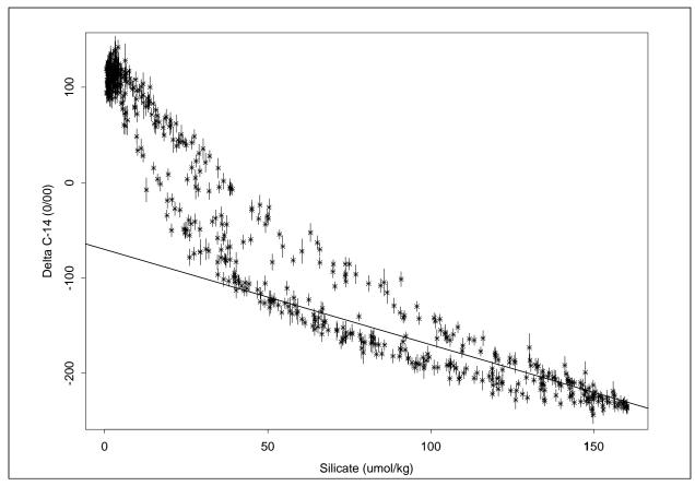
**Figure 3:**  $\Delta^{14}$ C as a function of silicate for P10 AMS samples. The straight line shows the relationship proposed by Broecker, *et al.*, 1995 ( $\Delta^{14}$ C = -70 - Si with radiocarbon in % and silicate in  $\mu$ mol/kg).
