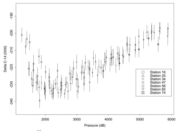
Figure 5: All LV  $\Delta^{14}$ C values as a function of pressure. Vertical bars indicate two sigma errors.
