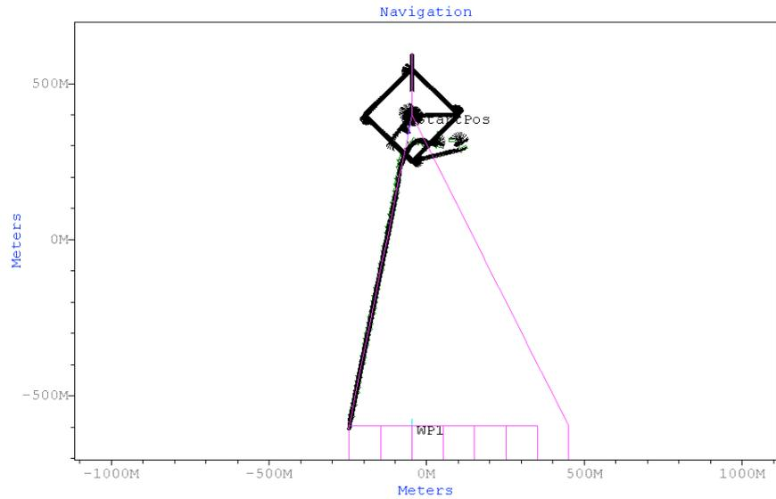
AUV-track (black) and mission profile lines for test dive 28. The mission was aborted shortly after the start of the first bottom line.
