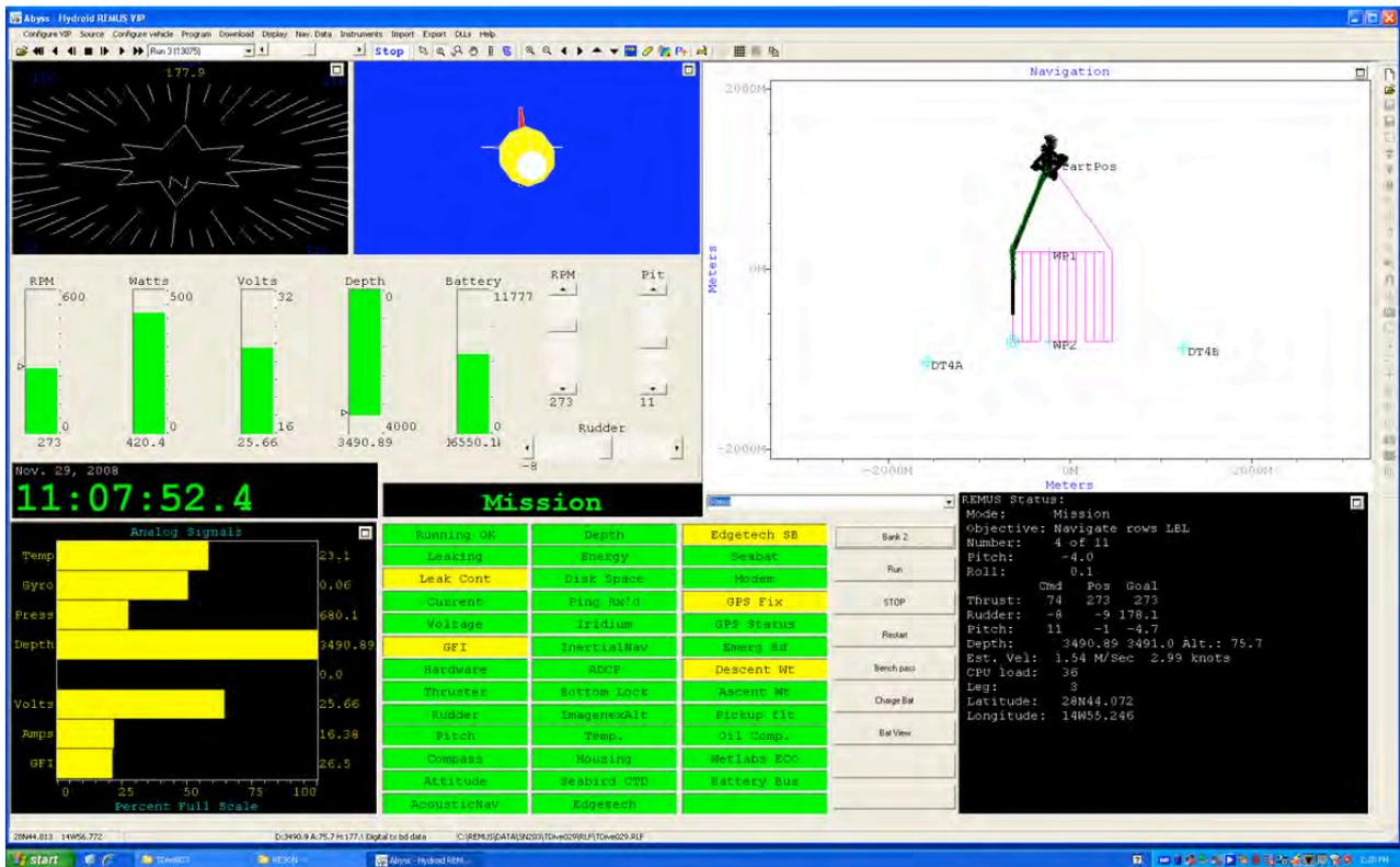
*Fig. 5: Screenshot of the Windows<sup>®</sup>-based vehicle interface program software (VIP) handling the AUV operations.*
