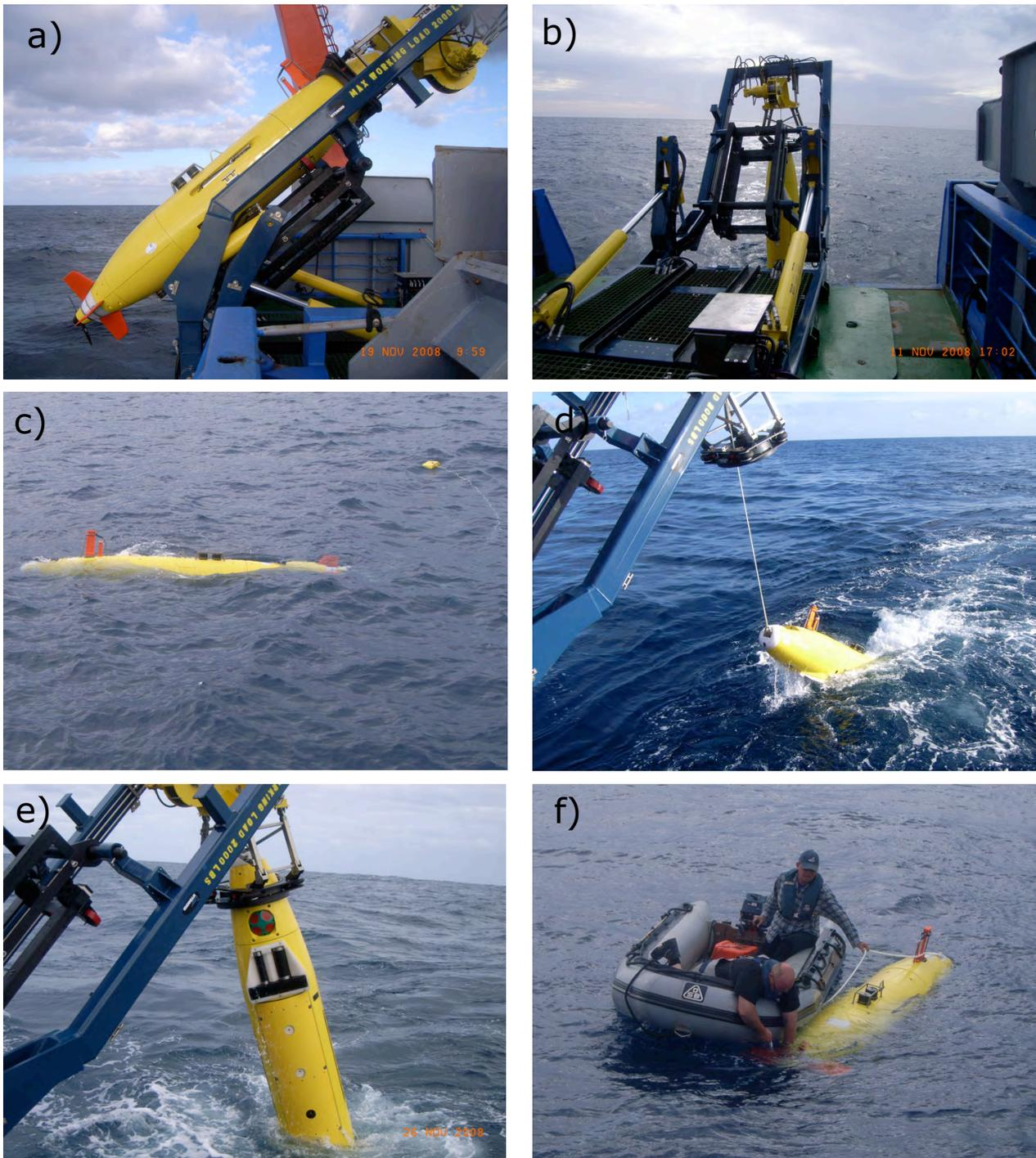
*Fig. 5: Details of the AUV ABYSS deployments. a) ABYSS shortly before launch, b) ABYSS is being launched, c) ABYSS after the mission; the pick-up float is released, d) Recovery with the LARS system, e) ABYSS connected to the LARS and being brought in, f) The zodiac had to be used after the recovery line was spun around the propeller of the vehicle.*
