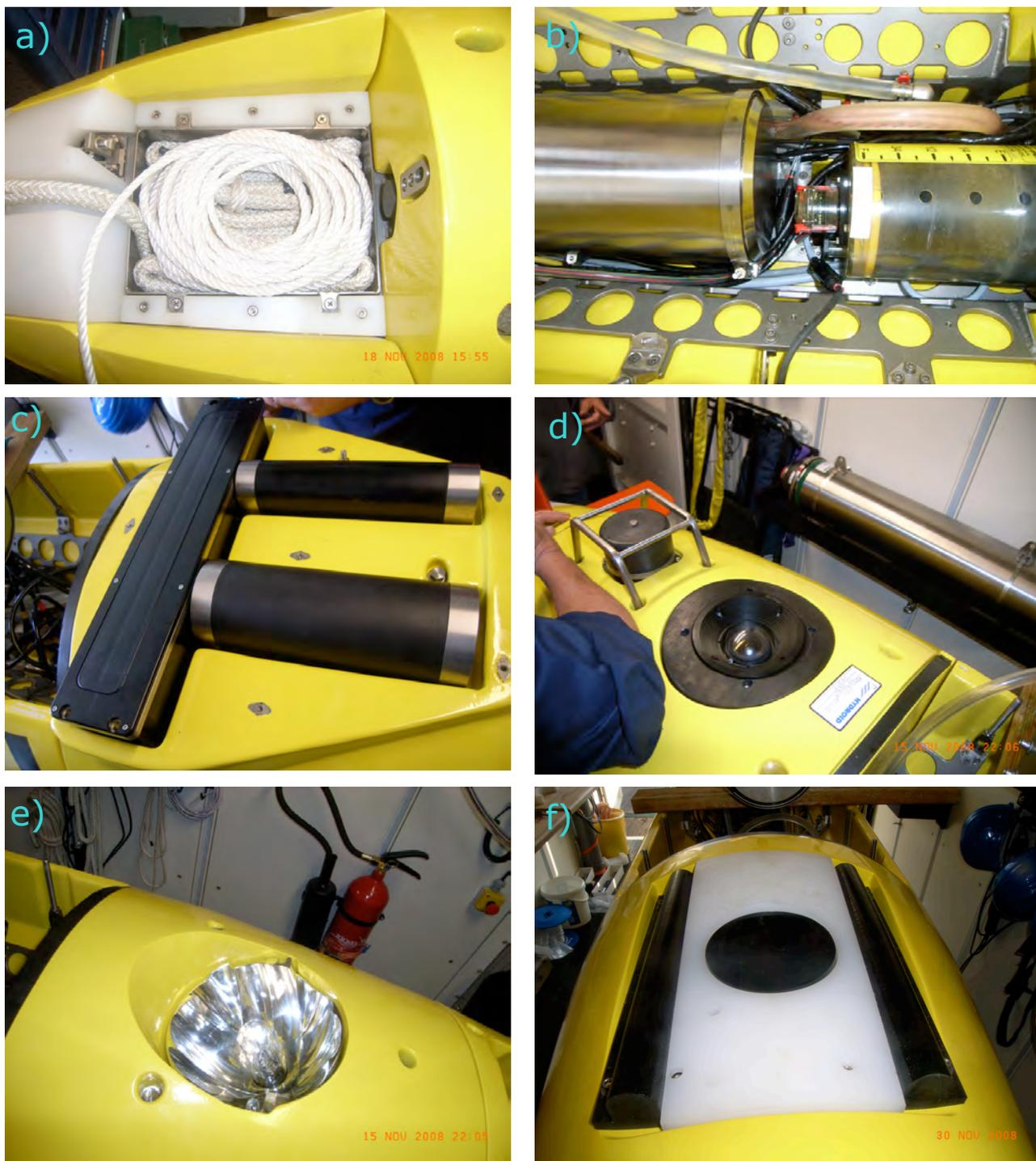
*Fig. 4: Details of the AUV ABYSS. a) view inside the pick-up float box, b) view inside the vehicle with main electronic bottle (left), oil compensator (right), and the titanium*
