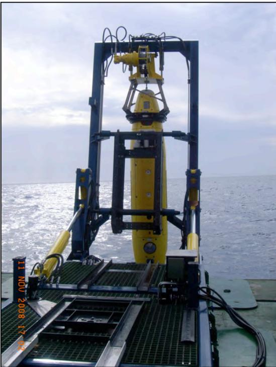
*Fig. 3: AUV ABYSS placed in its Launch- and recovery system (LARS).*
