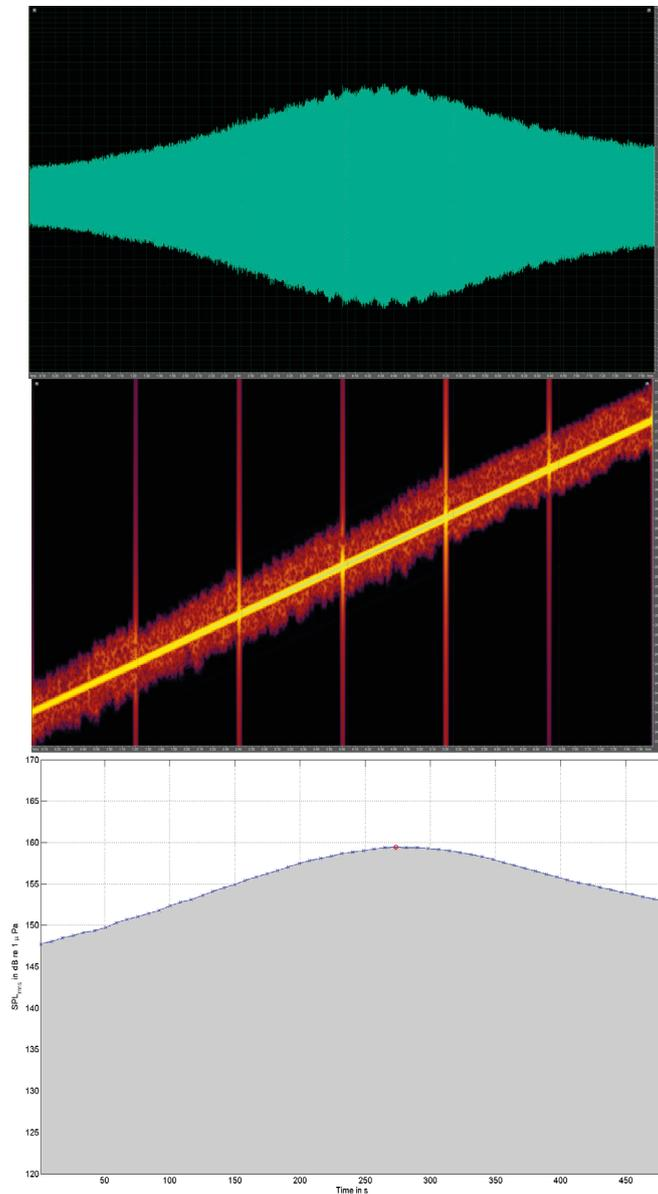
*Fig. 3.21: Frequency response of a RAFOS sound source. In each plot, the x-axis represents time in seconds since sweep start, being linearly related to sweep frequency. Top: Waveform of 6 collated 5-Hz sweeps. Middle: Spectrogram of collated waveform (broadband lines representing artifacts from the merging of files). Bottom: Relative sound pressure levels (arbitrary units) as function time (i.e. source frequency).*
