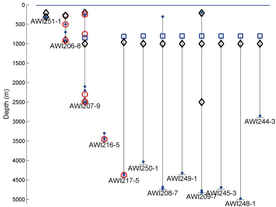
Fig. 3.5: Schematic of instrument distribution as hosted by moorings deployed across the Weddell Sea. Legend as in Figure 3.2; cyan cross: ADCP.
