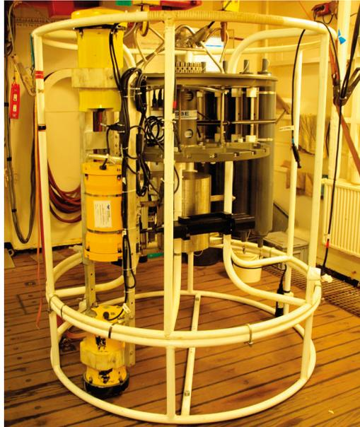
*Fig. 3.13: CTD and SBE32 carousel with RDI Workhorse Sentinels 300 kHz ADCP attached at the frame. The upward looking instrument (light yellow) is placed at the top, the downward looking instrument (dark yellow) at the bottom. The (slightly orange) unit in between is the housing for the extended battery pack.*
