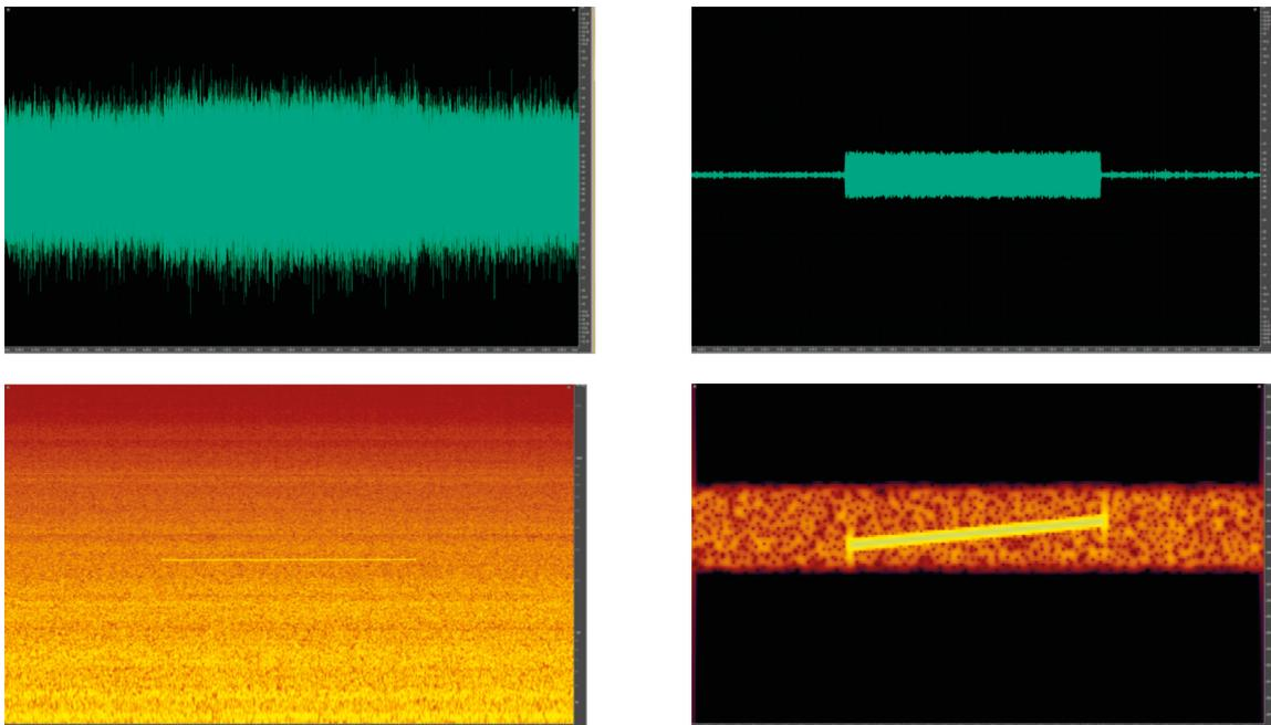
*Fig. 3.22: Waveforms and spectrograms recorded at 240 m depth of a RAFOS sweep produced by RAFOS sound source SN29 at 200 m depth.*
