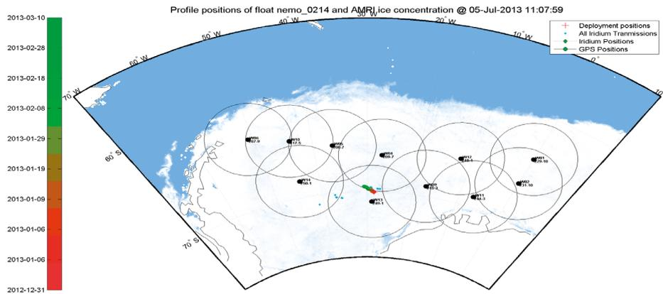
Fig. 3.16: Map of surfacing locations (red and green dots) of NEMO float S/N 214 deployed during ANT-XXIX/2 and ranges of RAFOS sound sources.
