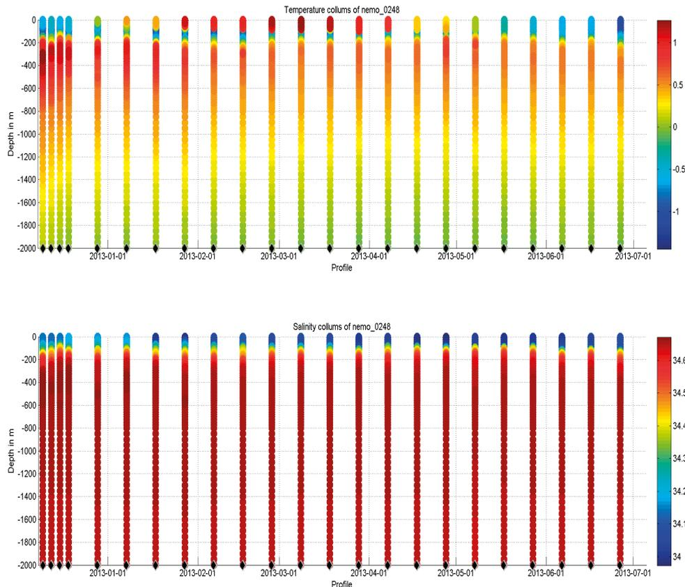
Fig. 3.15: Color coded temperature (top) and salinity (bottom) profiles from NEMO float S/N 248, approximately 7 months into its mission (profiles 1-23).
