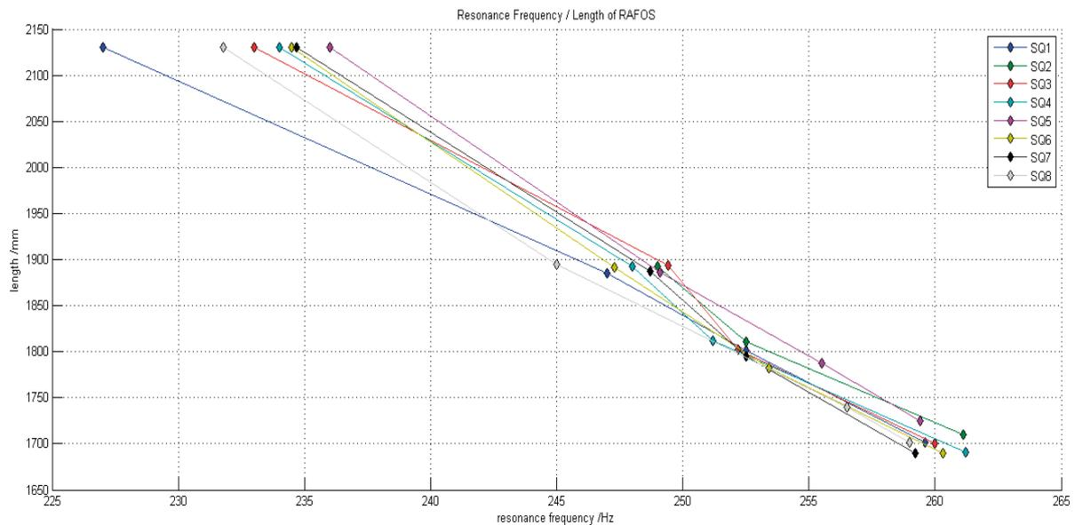
Fig. 3.23: Relation between resonance frequency and tube length for RAFOS sources.
