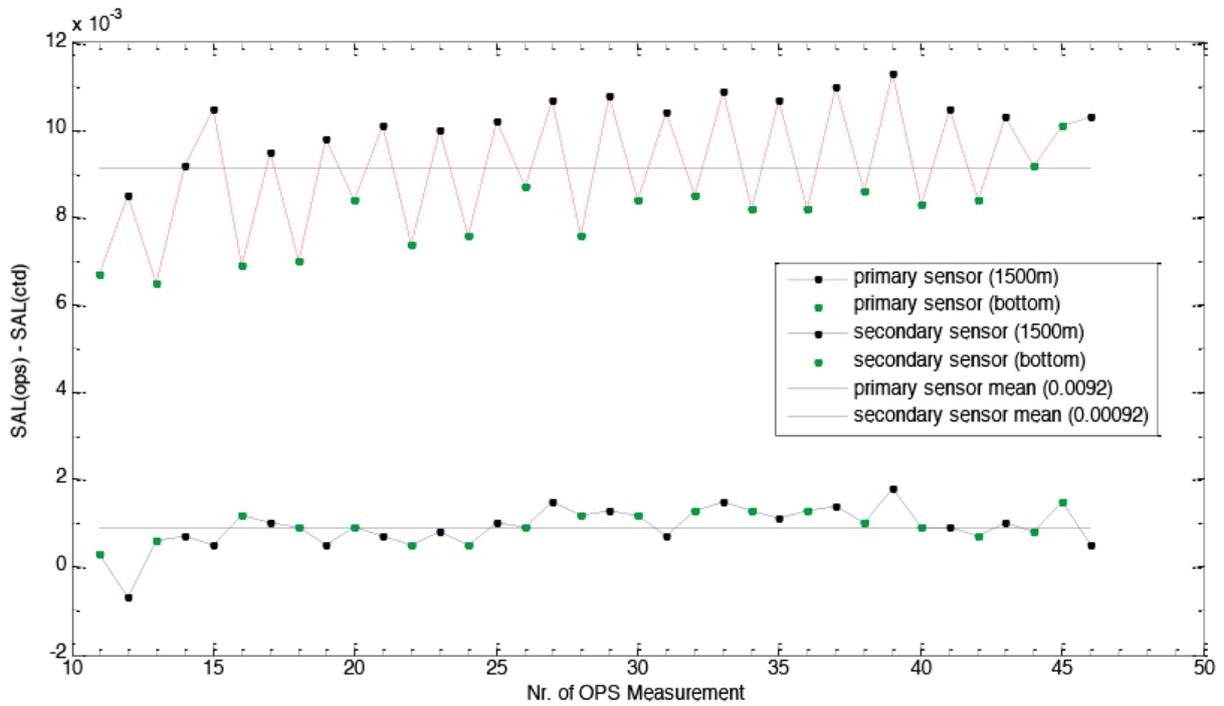
Fig. 3.10: Salinity deviations between OPS measurements and in-situ CTD measurements. The correction for the secondary sensor (black dashed line) is about  $0.0009 \text{ g}\cdot\text{kg}^{-1}$ , and lacked any discernible pressure dependency.
