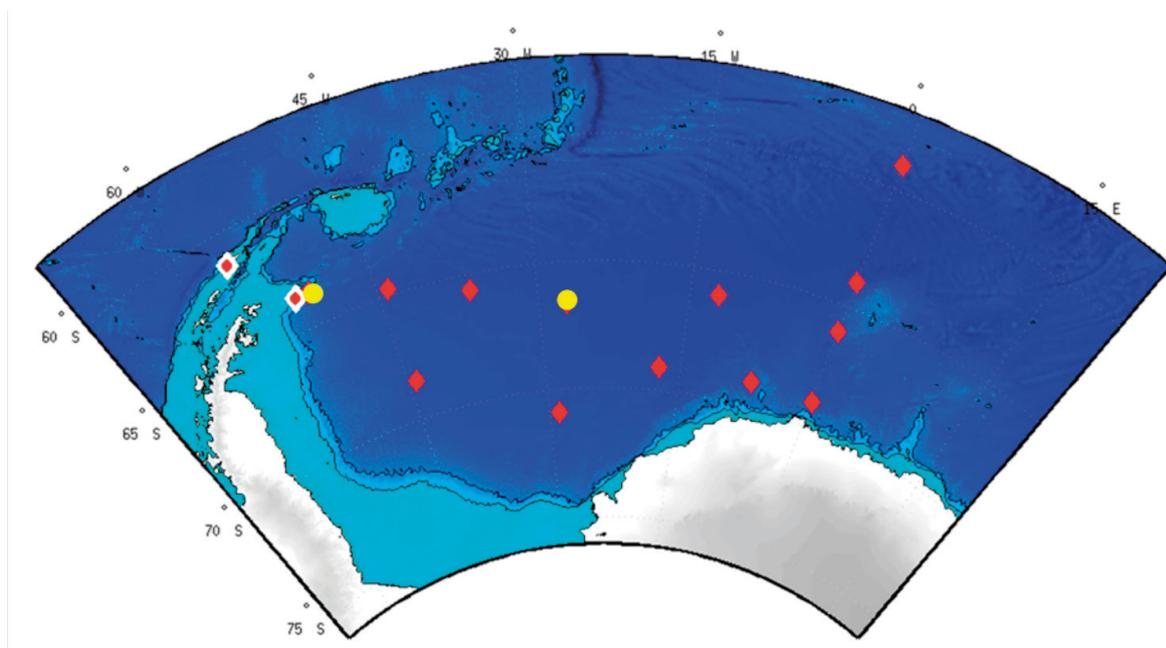
*Fig. 5.11: Map showing the locations where passive acoustic recorders were deployed during ANTXXIX/2. Red diamonds indicate positions where single SonoVaults were moored, yellow dots indicate moorings with three SonoVaults and red diamonds with a white outline indicate moorings with both an AURAL and a SonoVault.*
