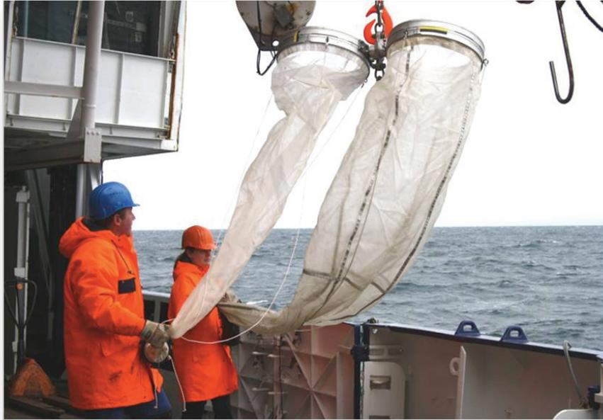
Fig. 4.2: Deployment of the Bongo net to collect zooplankton species
