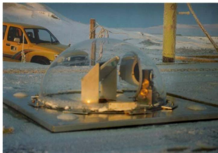
Figure 15 The tracker system of the Arrival Heights MAX-DOAS instrument.
