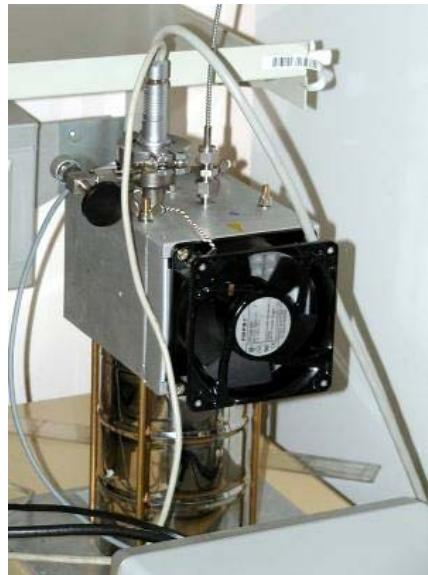
Fig. 6 New visible spectrometer installed in May 2002. Its telescope optics was integrated into the existing telescope set-up (see Fig. 5).
