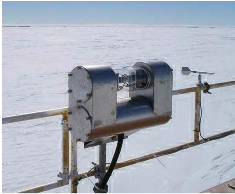
Fig. 14 New MAXDOAS telescope installed in early 2003. The Multi-Axis-Observations allow to infer more detailed information on tropospheric trace gases.
