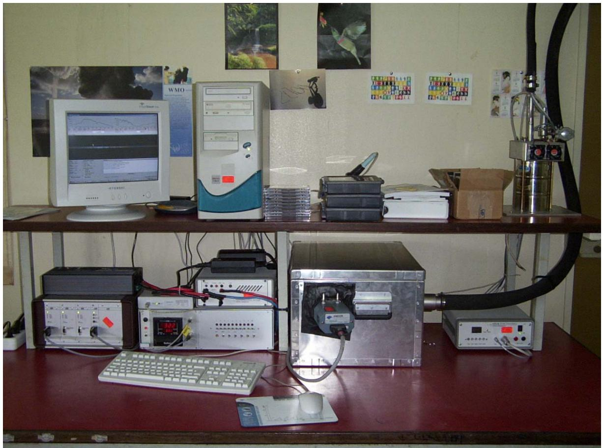
Fig. 10 Indoor set-up of the MAXDOAS instruments. The aluminium box at the bottom hosts the UV spectrometer; the small silver device at the right side of the board is the visible spectrometer.
