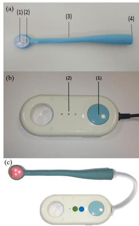
**Figure 1.** PetalB (Ptech Corp., Pyeongtaek, Republic of Korea). (a) Description of the laser irradiation part of PBMT device. (1) Laser irradiation unit; (2) laser irradiation part cover; (3) silicone handle; (4) main body connect port. (b) Description of the main body of PBMT device. (1) Device operation button; (2) operation indicator lamp. (c) Photos of laser being irradiated by connecting the main body and the laser irradiation part.
